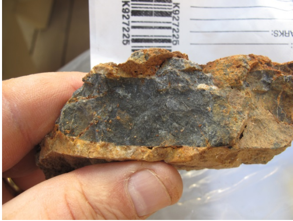
0.445 g/t Au, black carbonaceous schist cut by quartz-carbonate vein.
