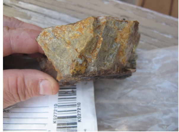
0.237 g/t Au in quartzite with limonitic fractures
