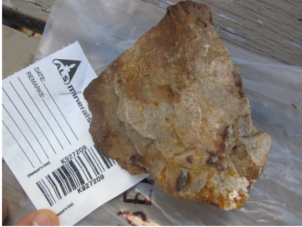
0.154 g/t Au in quartzite with arsenopyrite
