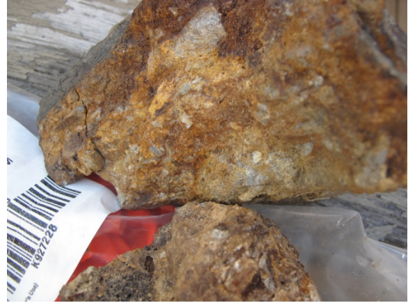
0.219 g/t Au in a brecciated quartzite with limonite matrix.
