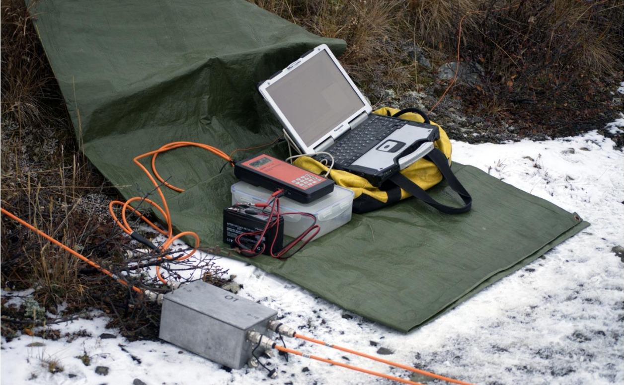
Figure 2 : 2D Resistivity measurement, Stefan Ostermaier, Arctic Geophysics Inc., Atlin, BC 2013
