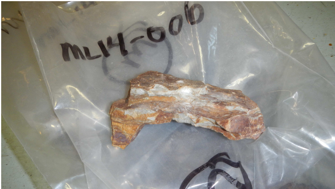
ML14-006 - f.g. Casca sandstone with f.g. Py – 775ppb Au
