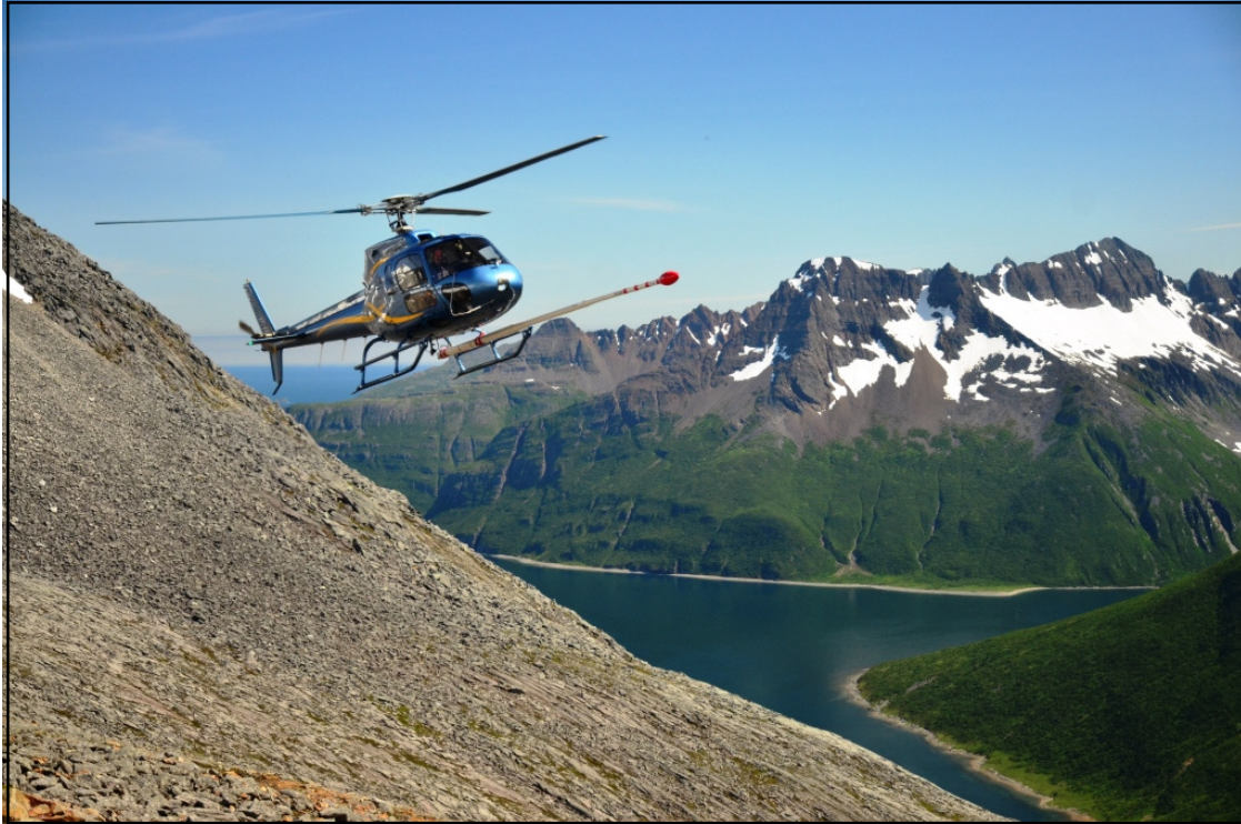
Figure 9: Eurocopter AS350 equipped with mag stinger for magnetic data acquisition, and internal spectrometer crystals for radiometric data acquisition.
