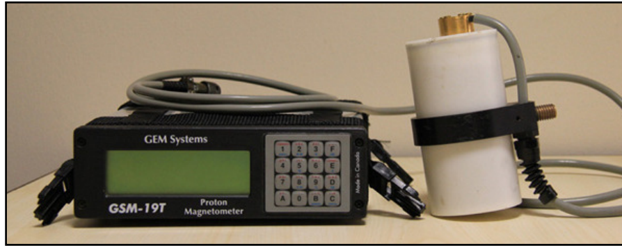
Figure 13: GEM GSM-19T proton precession magnetometer.
