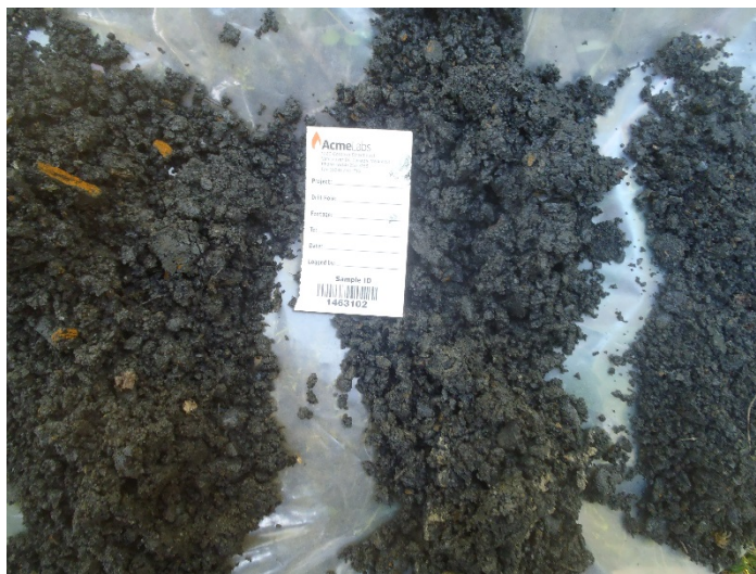
Figure 10: Typically elevated Mo in Nasina when rust is seen in graphitic black soil
