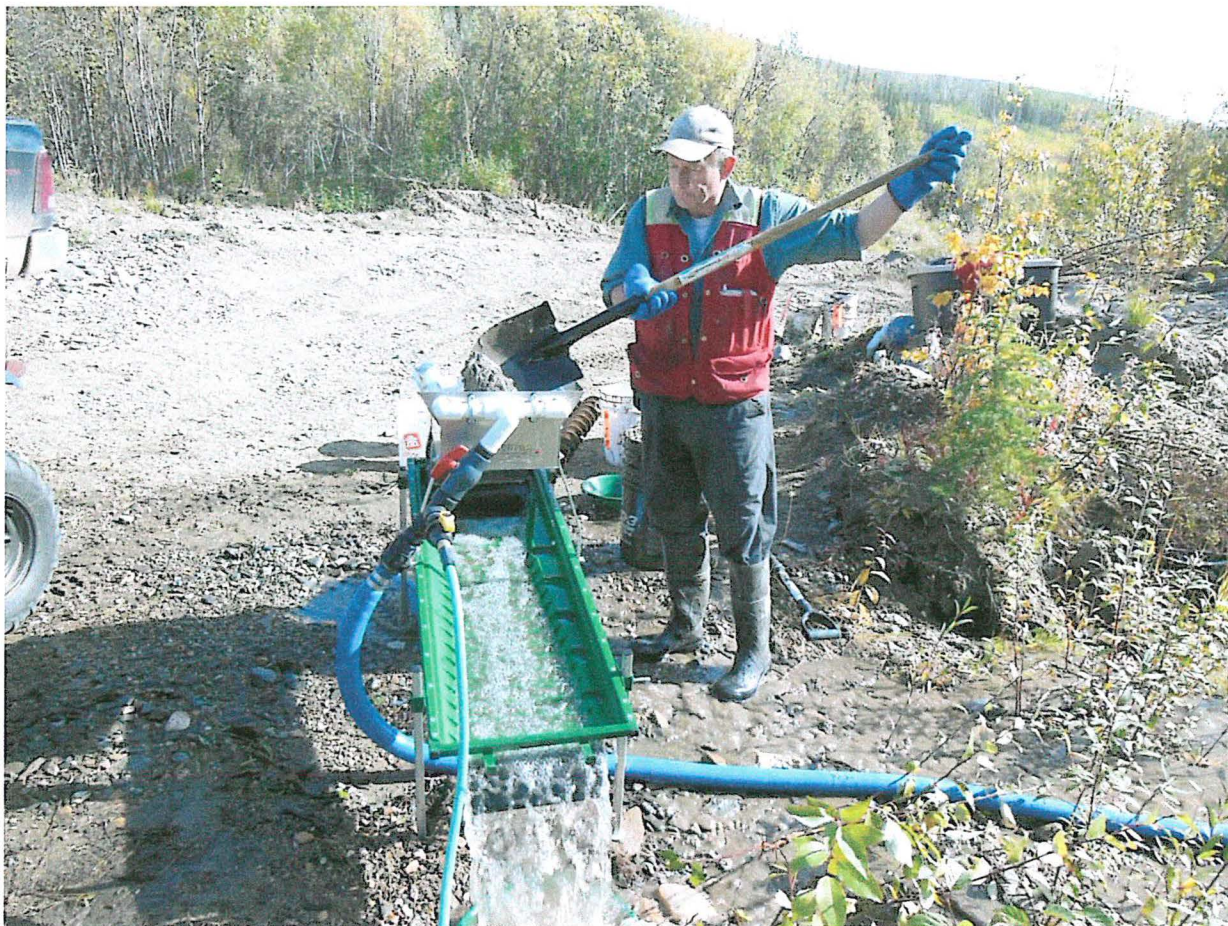
Plate 8 - The "Le Trap" sluice was fed through a wet hopper and screened to -1/4 inch. Riffles were easy to clean in-between samples and single-person operation was possible.
