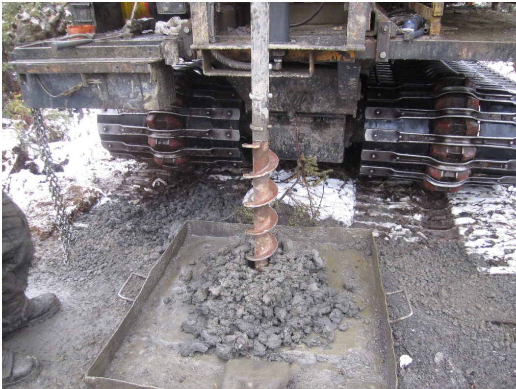
Photo 16: 6" Augers bringing up clumps of till into sample pan, hole M-38.
