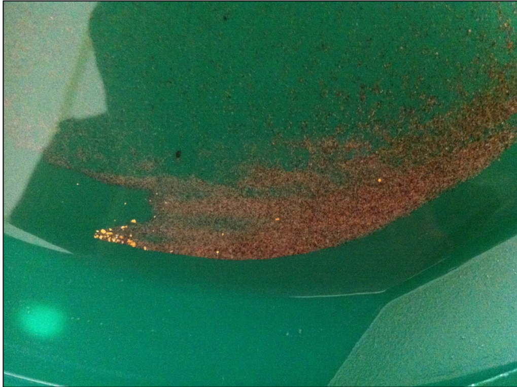
Figure 69. Gold recovered from just 0.3 loose cubic yard of a downstream bedrock dip (represent 2 ft gravel and 1 ft bedrock)
