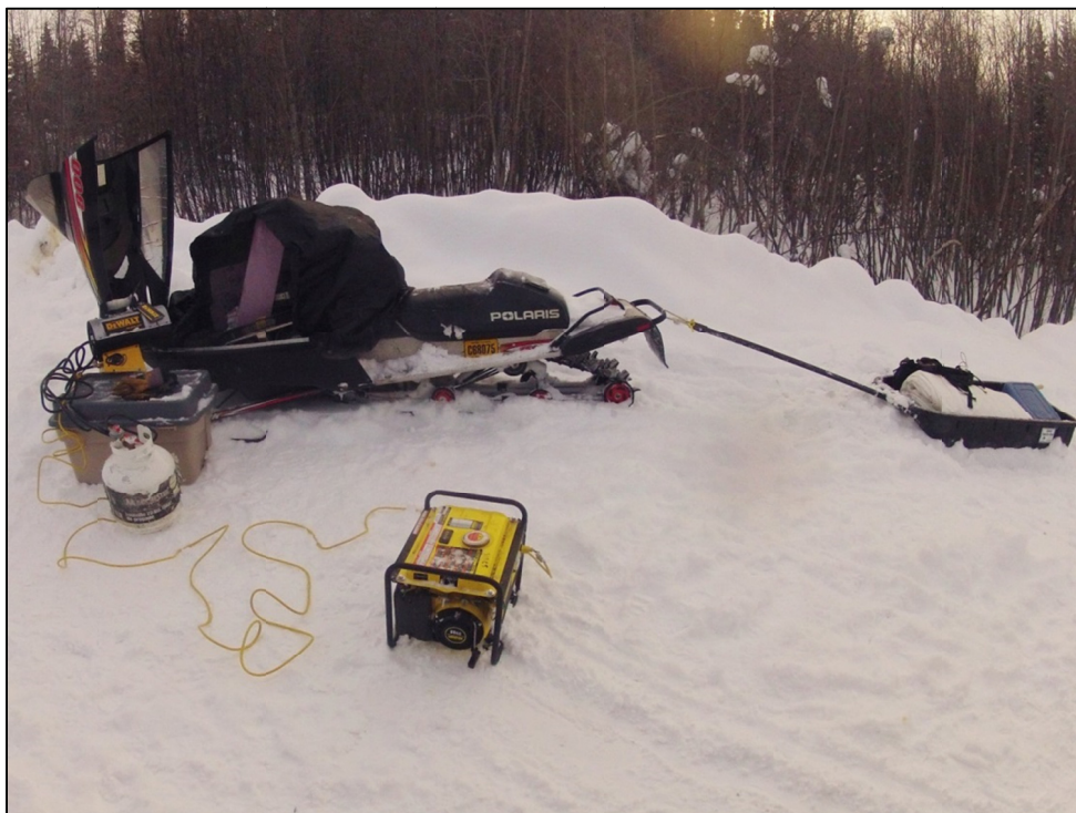
Figure 20. Using an electric generator to run a forced air propane heater to warm up the snowmobile engine in order to start in extreme cold
