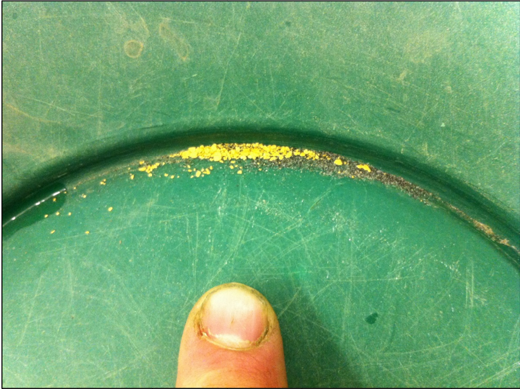
Figure 64. Gold recovered from 3.4 loose cubic yards sluiced of drift.
