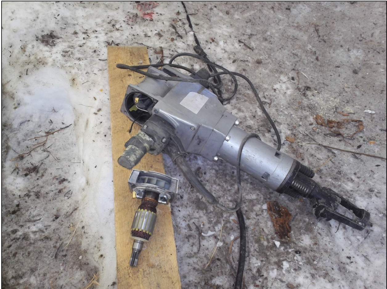
Figure 29. The brand new 100 lb (36 ft - lb) demolition hammer is out of service after less than 10 days of use.
