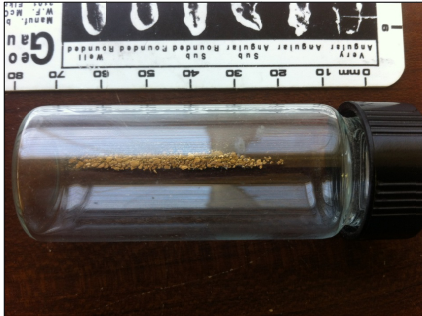
Figure 66. Gold recovered from 5.4 loose cubic yards of drift and chamber. The total raw gold weight is 0.365 grams.
