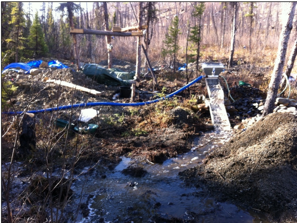
Figure 62. Shows the finer sand and silt (right) recovered from 3 cubic yards of sluiced drift
