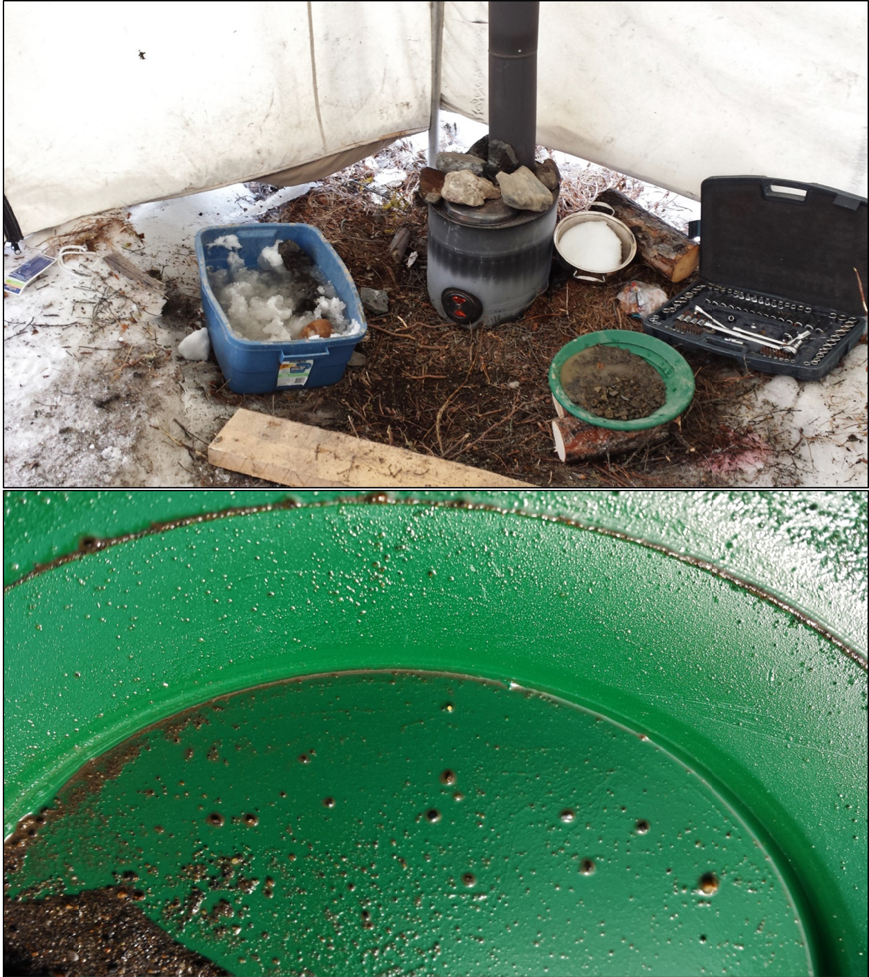
Figure 31. Upper photo shows melting water on the stove and thawing gravel in the pan. The lower photo shows a relatively course grain of gold recovered from a pan of gravel resting on bedrock (center of photo).
