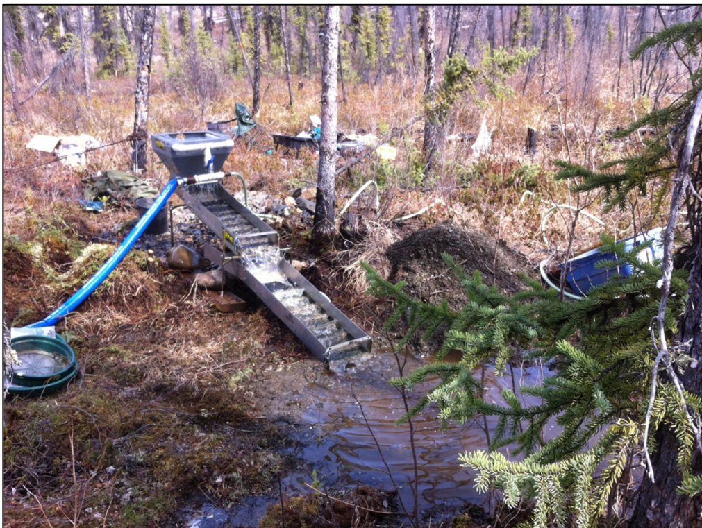
Figure 55. Sluce box setup.
