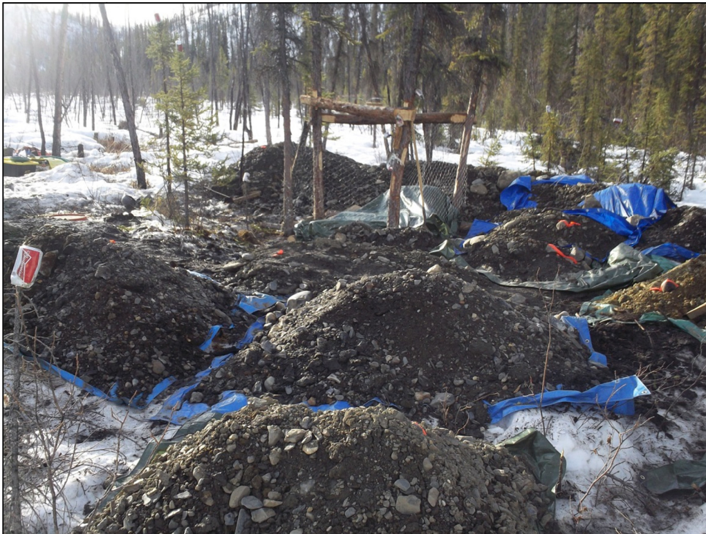
Figure 51. Stockpiled gravel for sluicing
