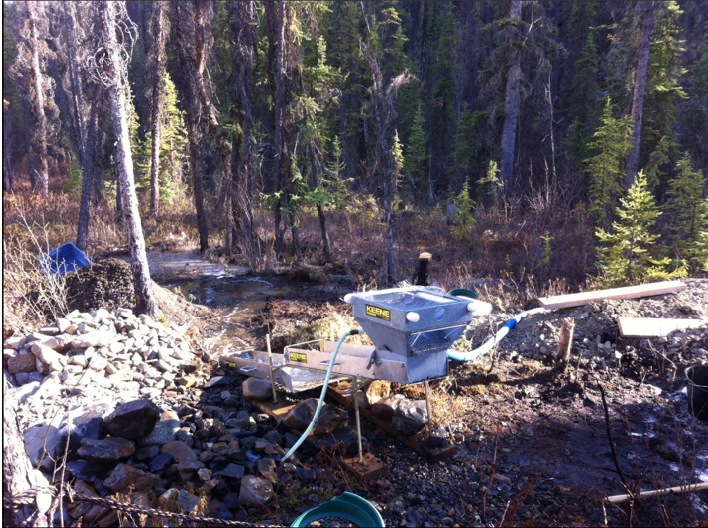
Figure 61. Shows boulders and cobbles (left) recovered from sluicing 3 cubic yards of drift
