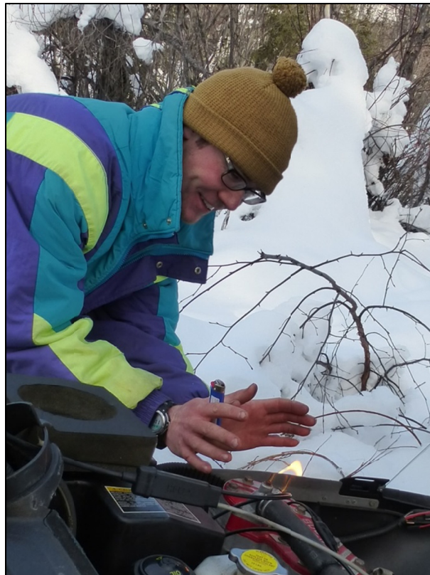
Figure 8. Burning the excess fuel in the snowmobile cylinders caused by the flooding carburetor.
