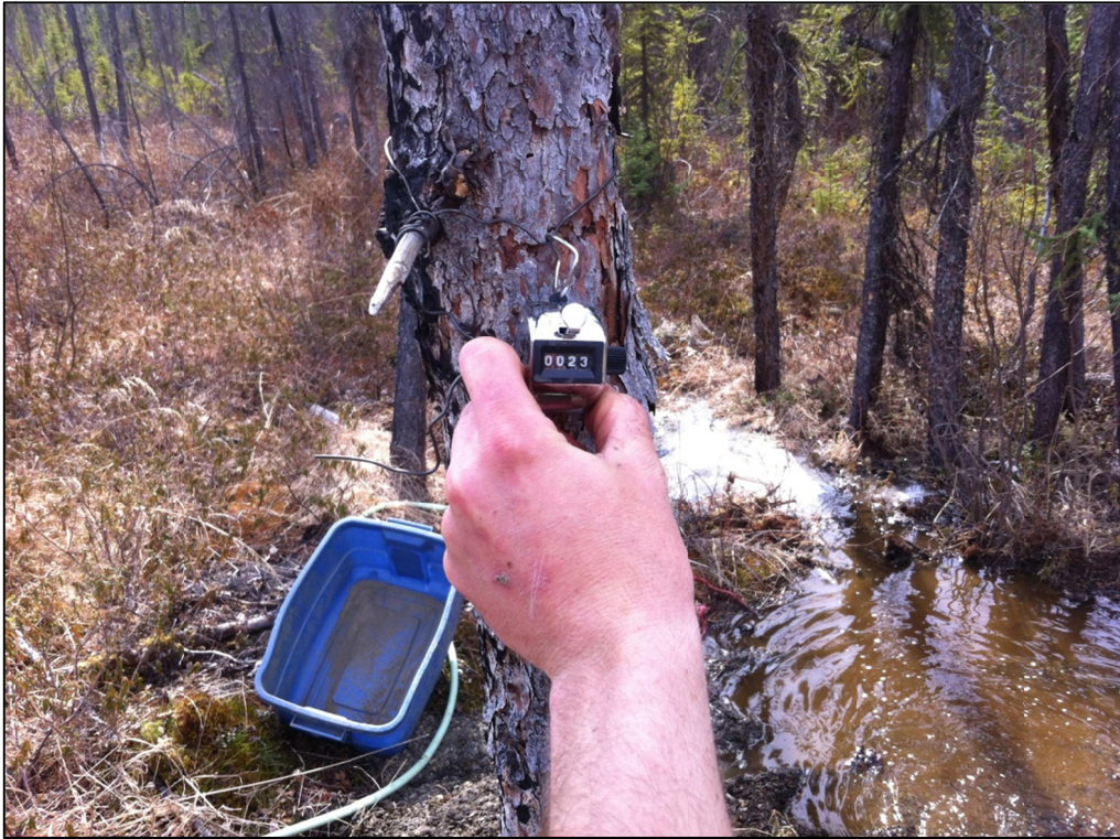
Figure 56. Counting device used to keep track of the number of buckets sluiced
