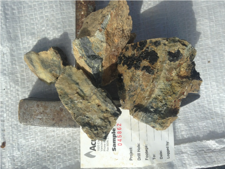
FIGURE 17 - MASSIVE ARSENOPYRITE AND QUARTZ VEIN MATERIAL FROM UPPER TREADWELL ADIT DUMP (12.1 G/T GOLD)
