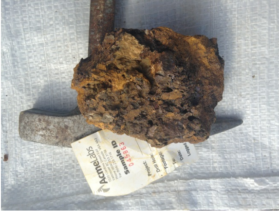
FIGURE 15 TRENCH DUMP SAMPLE SHOWING ROCK FRAGMENTS CEMENTED IN FAULT GOUGE
