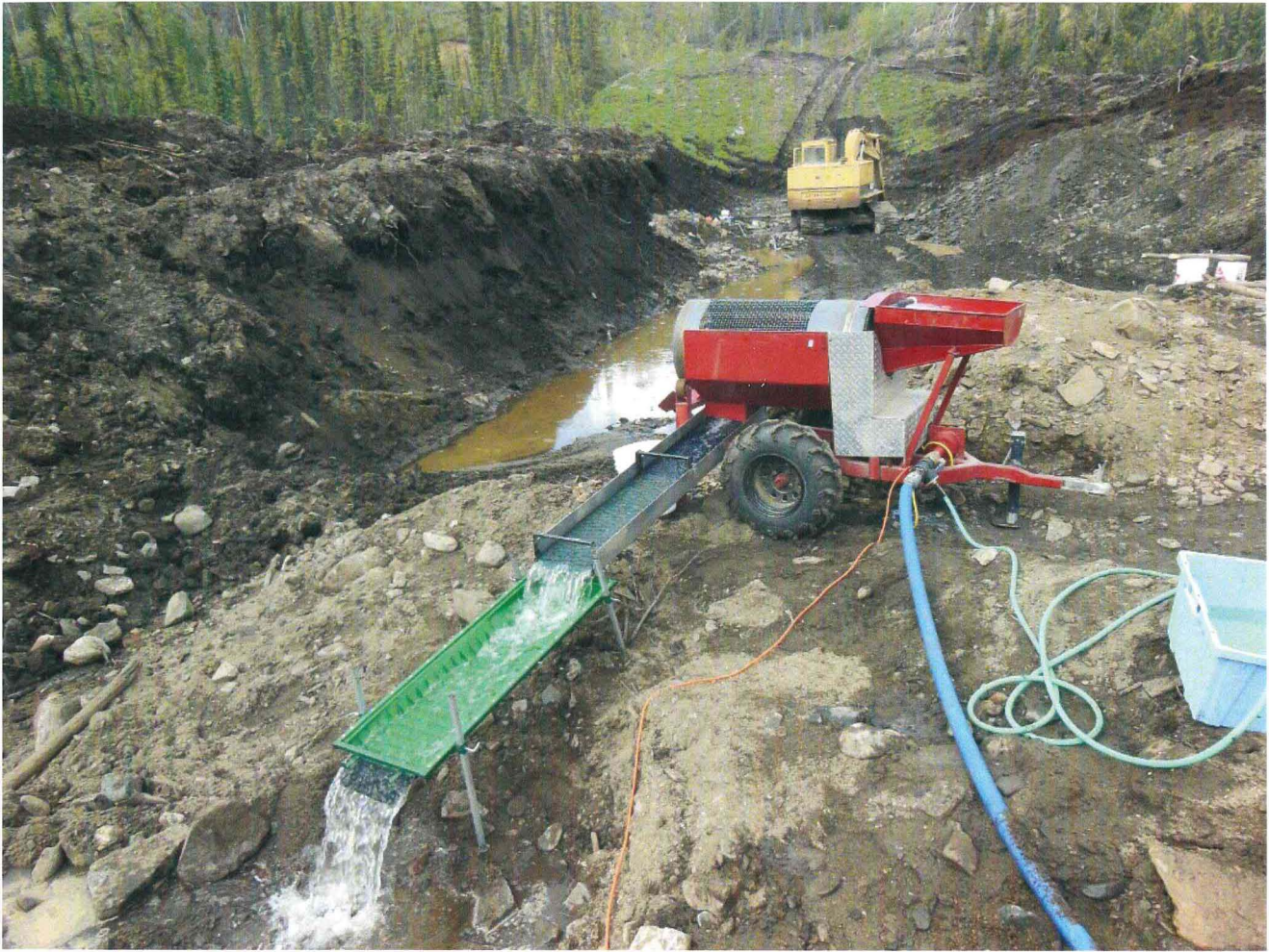
Plate 6 – The test trommel was mounted on an ATV-portable frame and had a \frac{1}{2} inch screen. Powered by an electrical motor with water supplied by a 1.5 inch pump, sluiced material was fed to a 6 foot aluminum sluice run with expanded metal riffles over unbacked Nomad matting, followed by 4 feet of a "Le Trap" sluice run.
