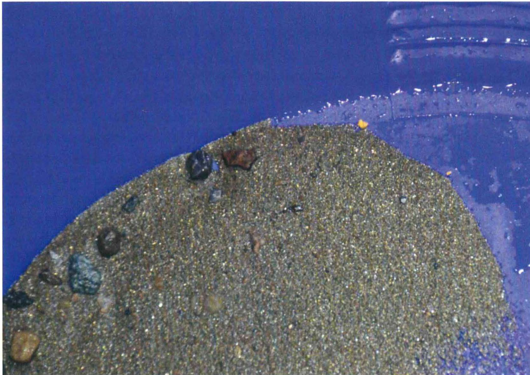
Plate 2 - Gold found in the BD-3 test pit in 2013 was "chunky" and tabular, not flat. Heavy minerals were a bi-modal mixture of fine-grained pyrite and coarse-grained magnetite, rutile, pyrite, garnet and scheelite.
