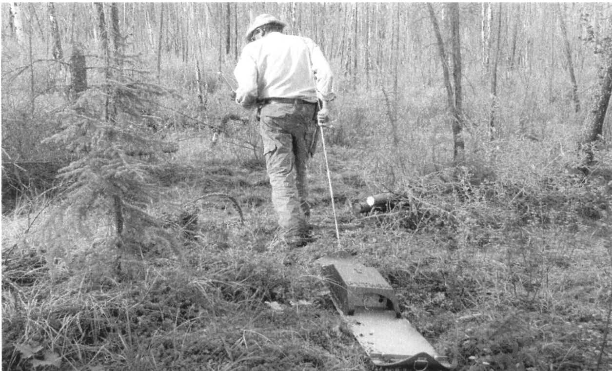
Figure 7. Surveys were conducted by using the Ground Penetrating Radar (GPR ) "Python".
