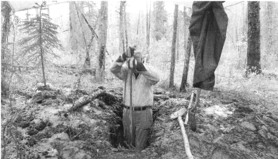
Figure 11. The testing Pit 1 at the Line #3 was stopped at top of permafrost zone.
