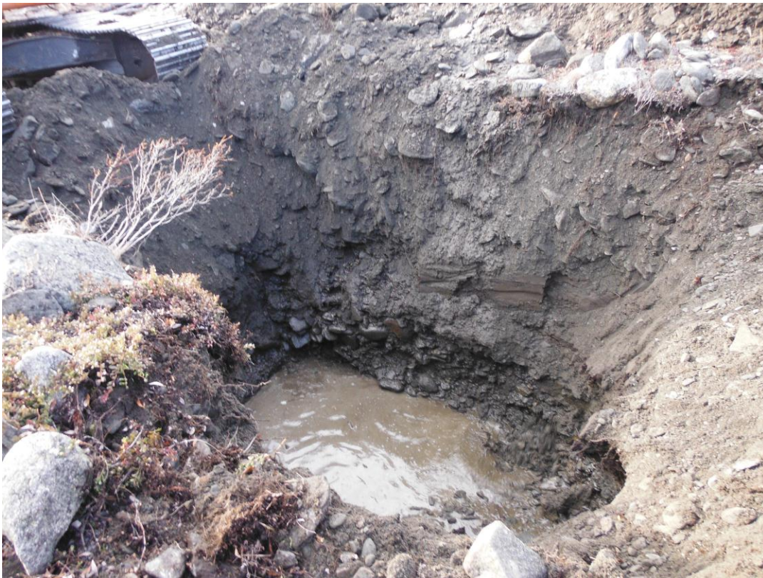
Figure 8: Test pit – Pits on lower Rabbit Creek and on Larose Creek filled with groundwater between 10-15 ft.
