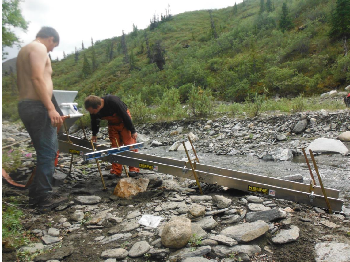
Figure 9: Setting up the Power Sluice.
