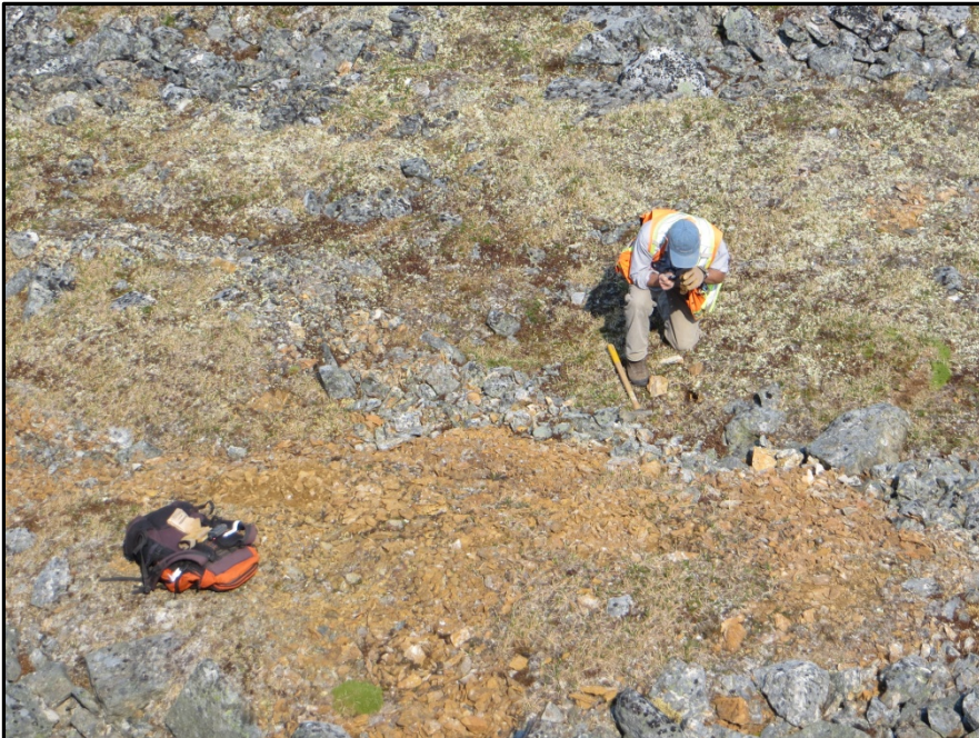
Camp 2, Soil sample site 579478. Limonite – carbonate altered andesite in frost boil, likely a fault zone.
