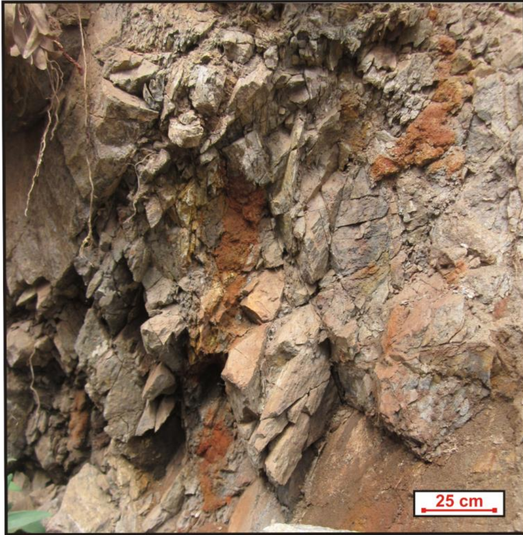
Figure 5.4-6 Typical outcrop texture of intensely fractured Station Creek rocks. Iron oxide discolouration is a common attribute of these brittle structures.
