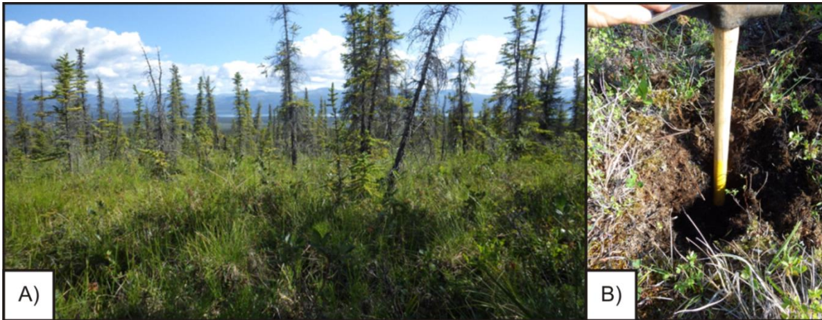
Figure 6.4-12 A) Typical terrain in areas of M7, M8, and M9. B) A test soil pit with permafrost encountered at approximately 25 cm depth.
