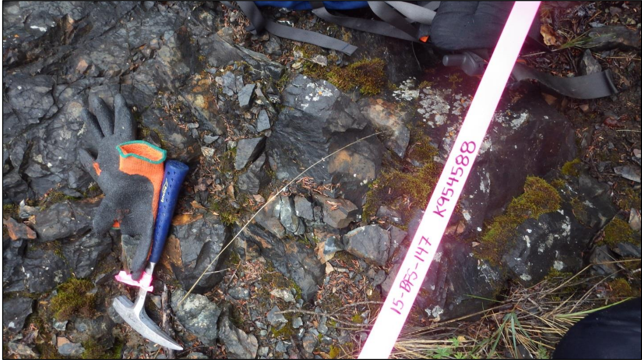
Figure 6.3-24 Outcrop of peridotite and sample K954588 which returned the highest platinum (83.5 ppb), highest palladium (175.1 ppb) and second highest chromium (5952 ppm) values of all the rock samples analyzed from Phase 1. Other elements were also enriched; 1759.3 ppm nickel and 150.7 ppm cobalt.
