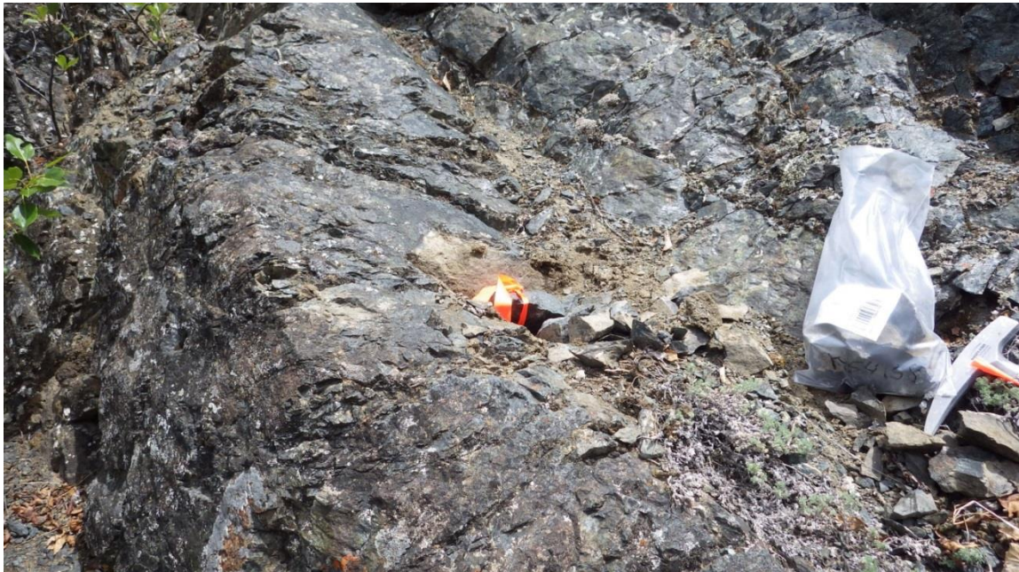
Figure 6.4-1 Massive, fine to coarse grained, moderately to strongly magnetic, very dark green to black ultramafic rock within M11 and 12.
