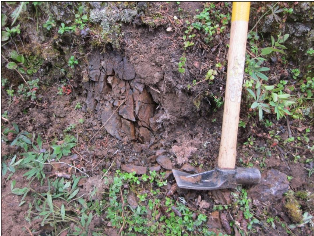
Figure 6.4-15 Non-magnetic, dark grey to black (and slightly gossanous) argillite found in the southeastern extent of M13 (K954587).
