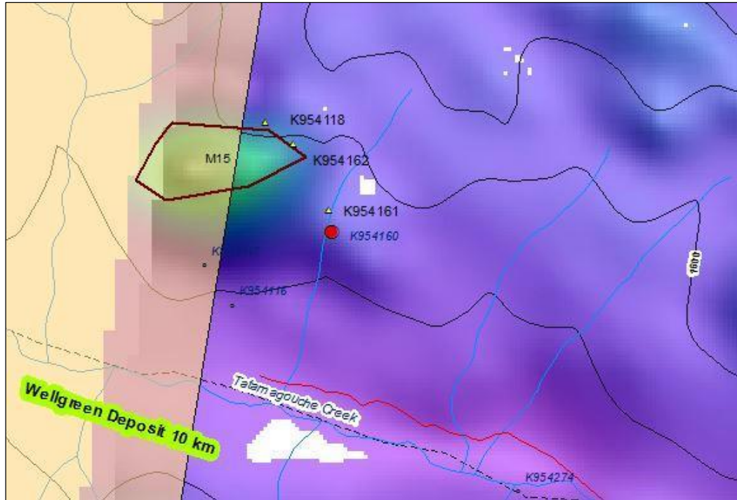
Figure 6.4-6 Target M15, showing relative cobalt values for rocks (triangles) and streams (circles). Stream sediment sample K954160 is elevated in Co, Cr, Ni, Cu and Ag.
