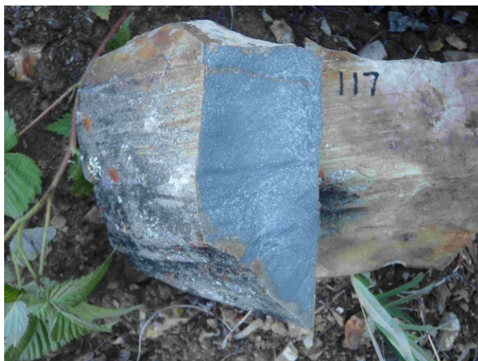
Fig. 4. Biotite hornfels alteration. Massive texture with conchoidal fracture on fresh surface with remnant banding visible on the weathered surface.
