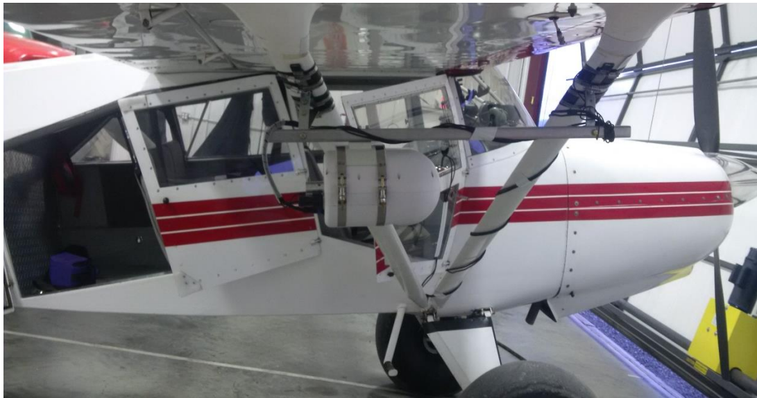
Figure 19: The pod secured the bar attached to the strut.
