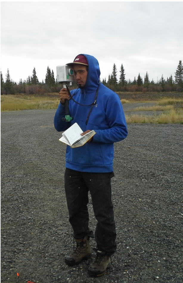
Figure 9: Operating the EM-16 VLF-EM machine. Fieldbook is used to record readings.
