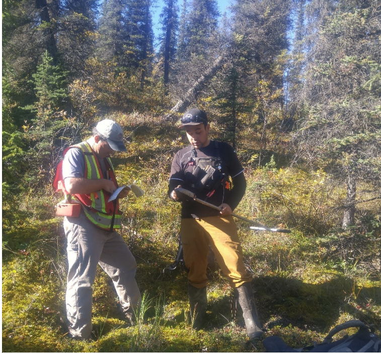
Figure 10: Contour soil sampling west of the Duke River. One person collects the sample using the Dutch auger while the other records location and sample description.
