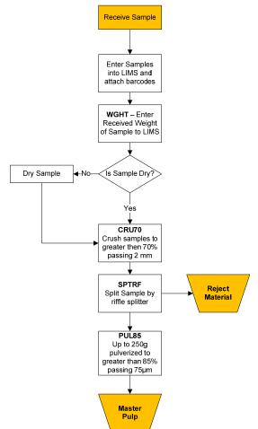
Received samples are entered into the Laboratory Information Management System (LIMS), weighed, dried and crushed to ensure that greater than 70% pass a 2mm sieve. A 250g split of the crushed material is then pulverized to greater than 85% passing a 75 $\mu$ m sieve.
