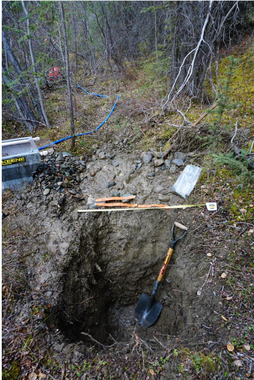
Plate 5 - Test Pit Max #3 encountered an organic rich sand overlying a sandy gravel.
