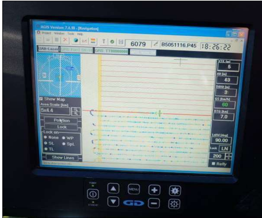
Figure 11: AGIS operator display installed in the Eurocopter AS350, with screen displaying real time flight line recording and navigation parameters. Additional windows display real time geophysical data to operator.
