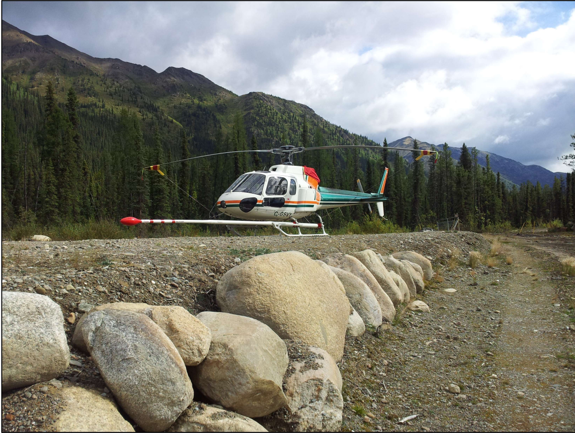
Figure 12: View of the mag stinger used on the Seattle Creek survey.
