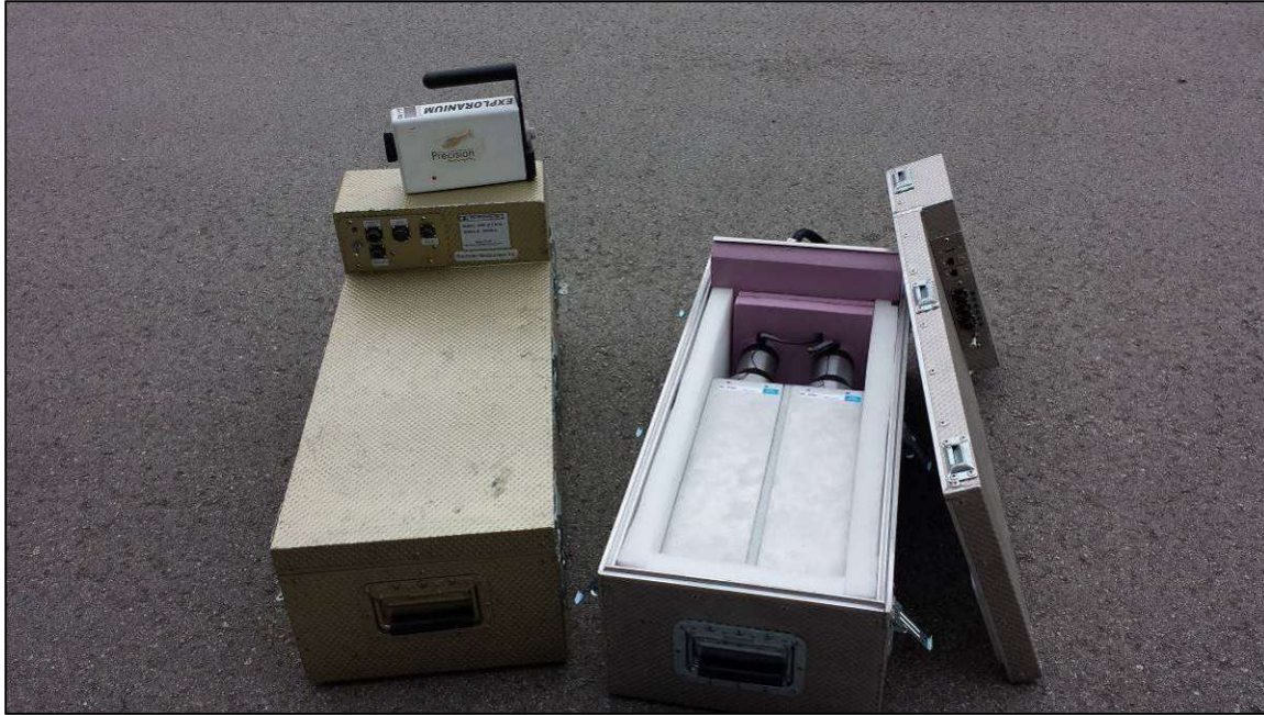
Figure 13: GRS-10 Thallium-activated Sodium Iodide gamma spectrometer crystal pack. The open unit on the right shows two individual 4.2 liter detectors.
