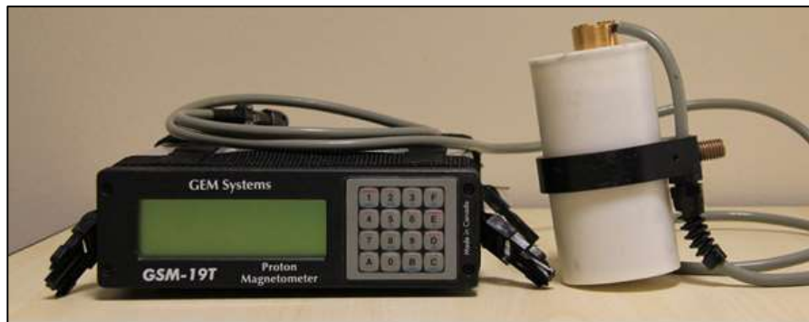
Figure 14: GEM GSM-19T proton precession magnetometer.
