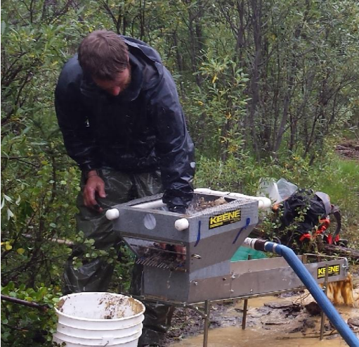
Photos 4 and 5: Running the drill cuttings through a sluice and panning the concentrate.
