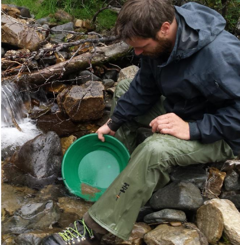
Photos 4 and 5: Running the drill cuttings through a sluice and panning the concentrate.
