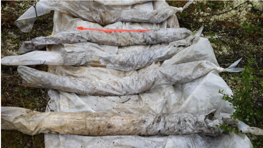
Photo 3: 5 ft runs laid out for logging.
