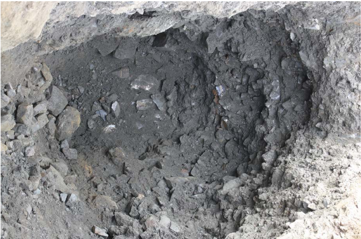
Figure 28: TP-1 Rocky Till at bottom of pit. img 4093
