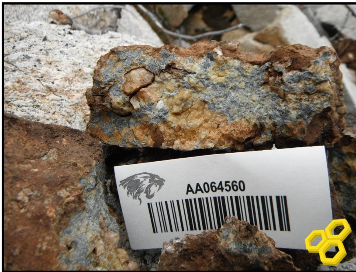
Figure 9.1. Example of scorodite vein at surface. Sample AA064560 has an assay grade >25g/t Au.
