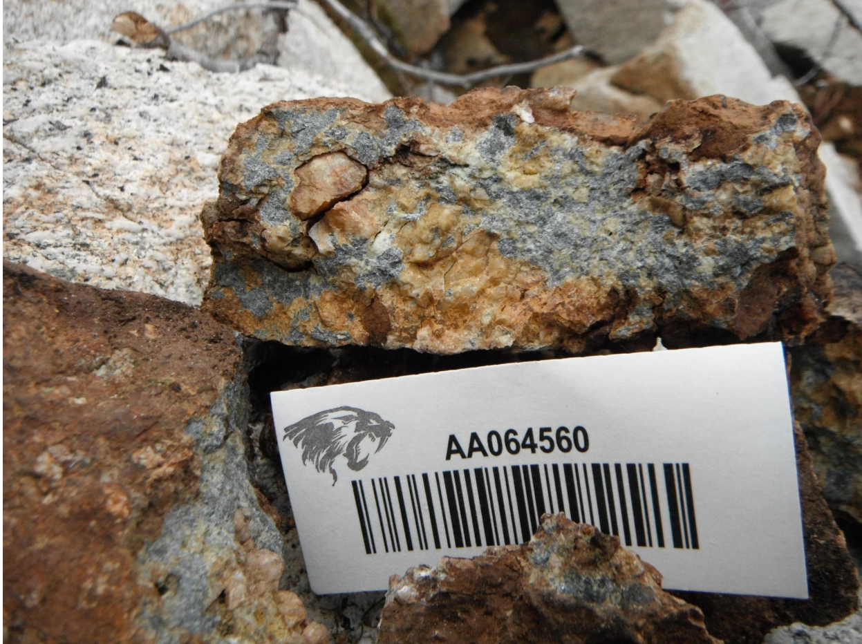
Figure 8.1 Example of scorodite vein at surface. Sample AA064560 has an assay grade >25g/t Au.
