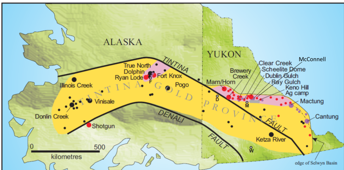
Figure 7.1 Map of the Tintina Gold Province for the Yukon Territory and Alaska. Mineral deposits are shown as large circles, mineral occurrences are shown as small circles. Gold deposits in red dots could be considered under the same genetic model as McConnells Jest. Deposits marked in black dots are not of the same origin, or are ambiguous in origin. Deposits marked in purple are skarn deposits (predominantly W-bearing). Within the TGP is the Tombstone Gold Belt (TGB; marked in pink) which is the major host to gold deposits in the Yukon and Alaska. Mair et al. (2006) suggested ~450 km of post-formation offset along the Tintina Fault, causing displacement of the Fairbanks district. Population centres marked are Whitehorse (W), Mayo (M), Dawson (D) and Fairbanks (F). After Hart (2007).
