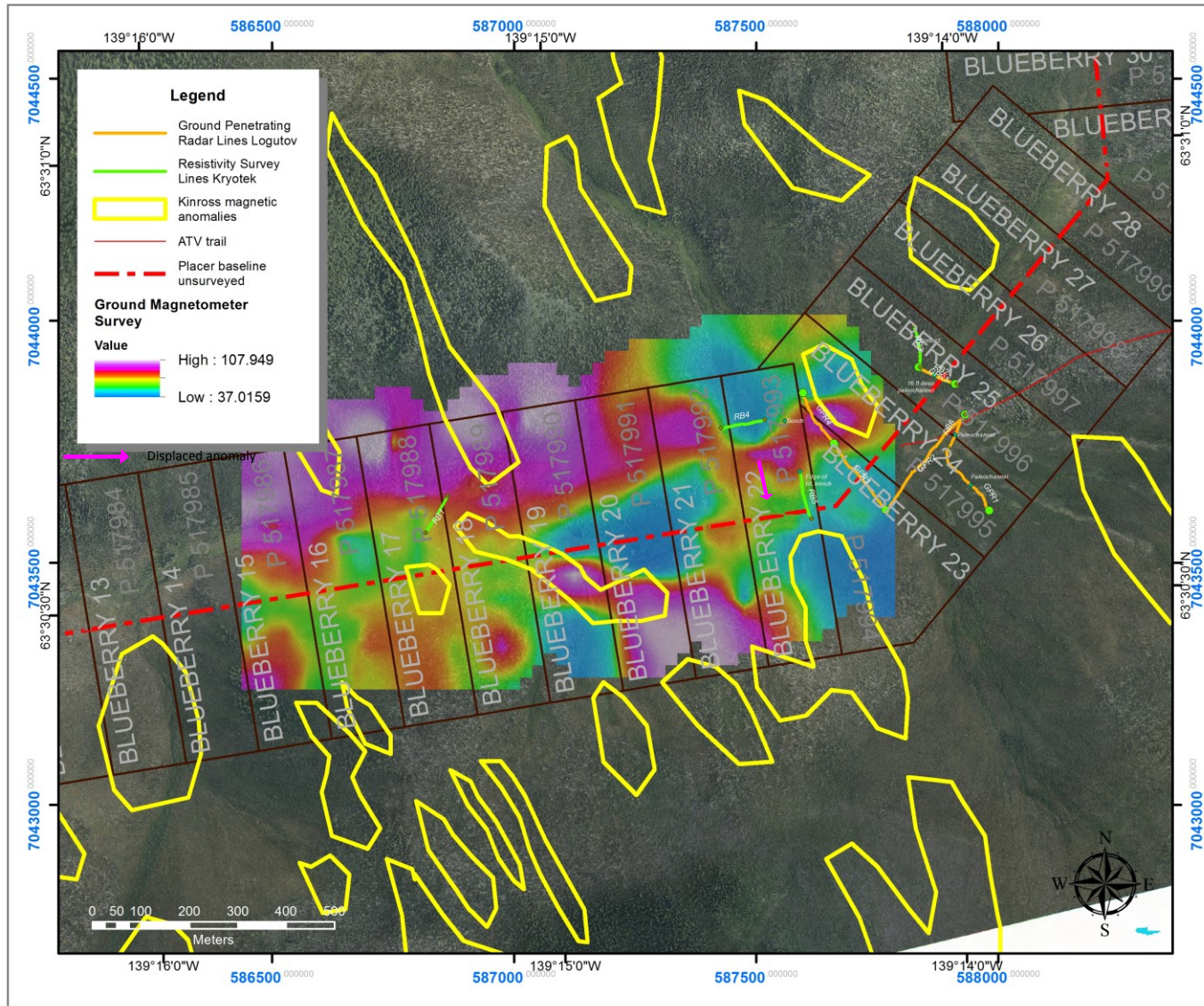
Figure 13 – Compilation map of 2016 exploration program on Rosebute Creek, showing Kinross regional magnetic anomalies (Hollis, 2011) overlain on the 2016 ground magnetometer survey. The locations of the ground penetrating radar lines and resistivity survey lines are also shown.
