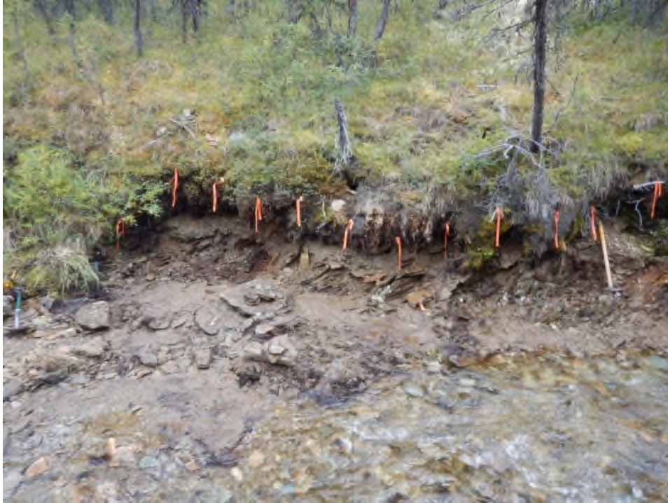
Figure 15. North Baldy Showing and adjacent outcrop. Mineralization, largely covered by colluvium, occurs in stripped area near left (southeast) side of photo. Orange flags are spaced 0.5 m apart. View towards 220°.
