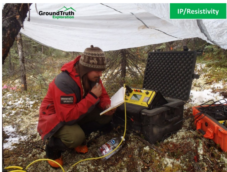
Figure 7 – Supersting DC IP-Resistivity system.
