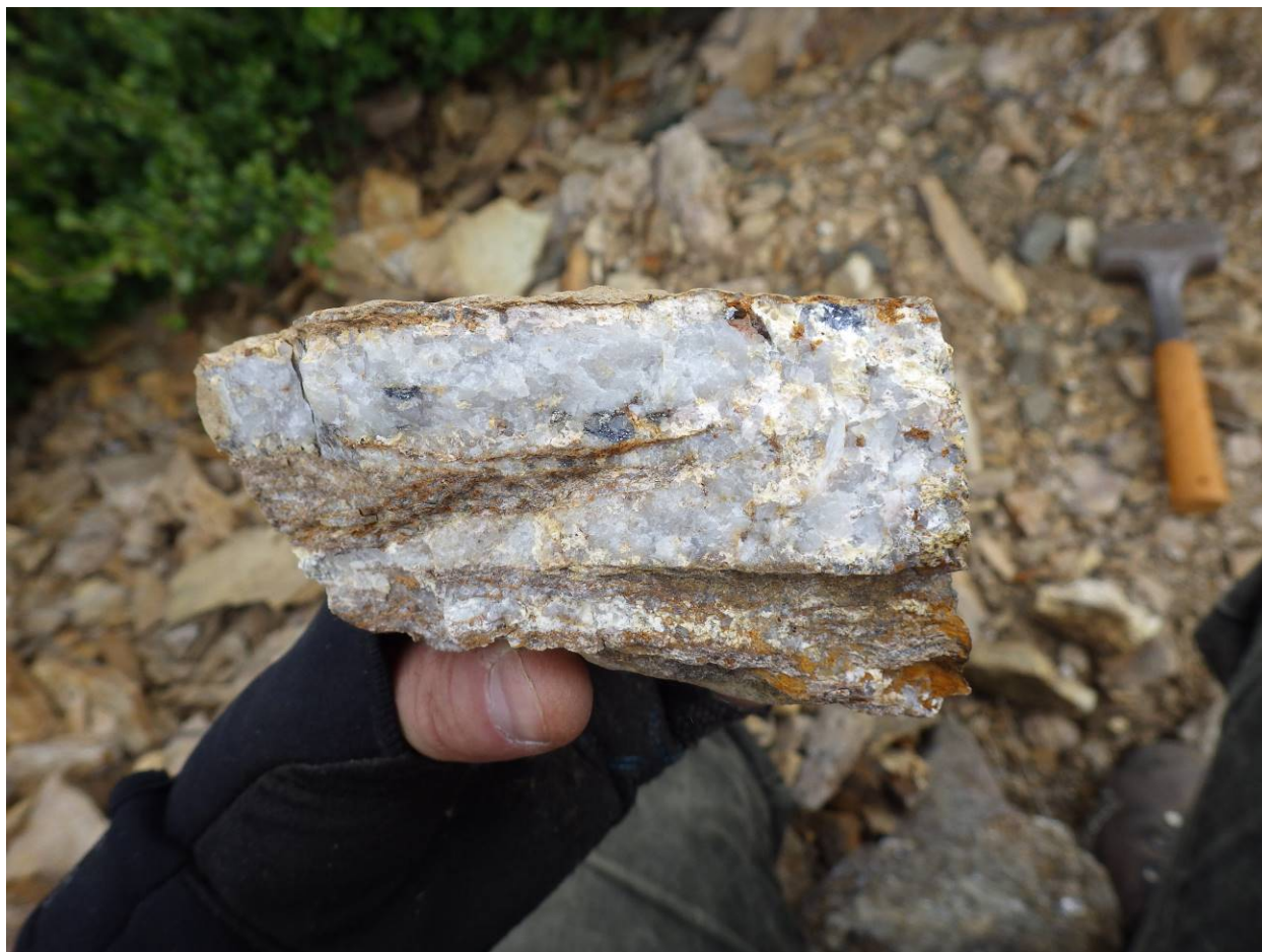
Figure 22: Galena bearing quartz vein from NW Zone. Sample 1426312; assayed 1.49 g/t Au & 693 ppm Pb.
