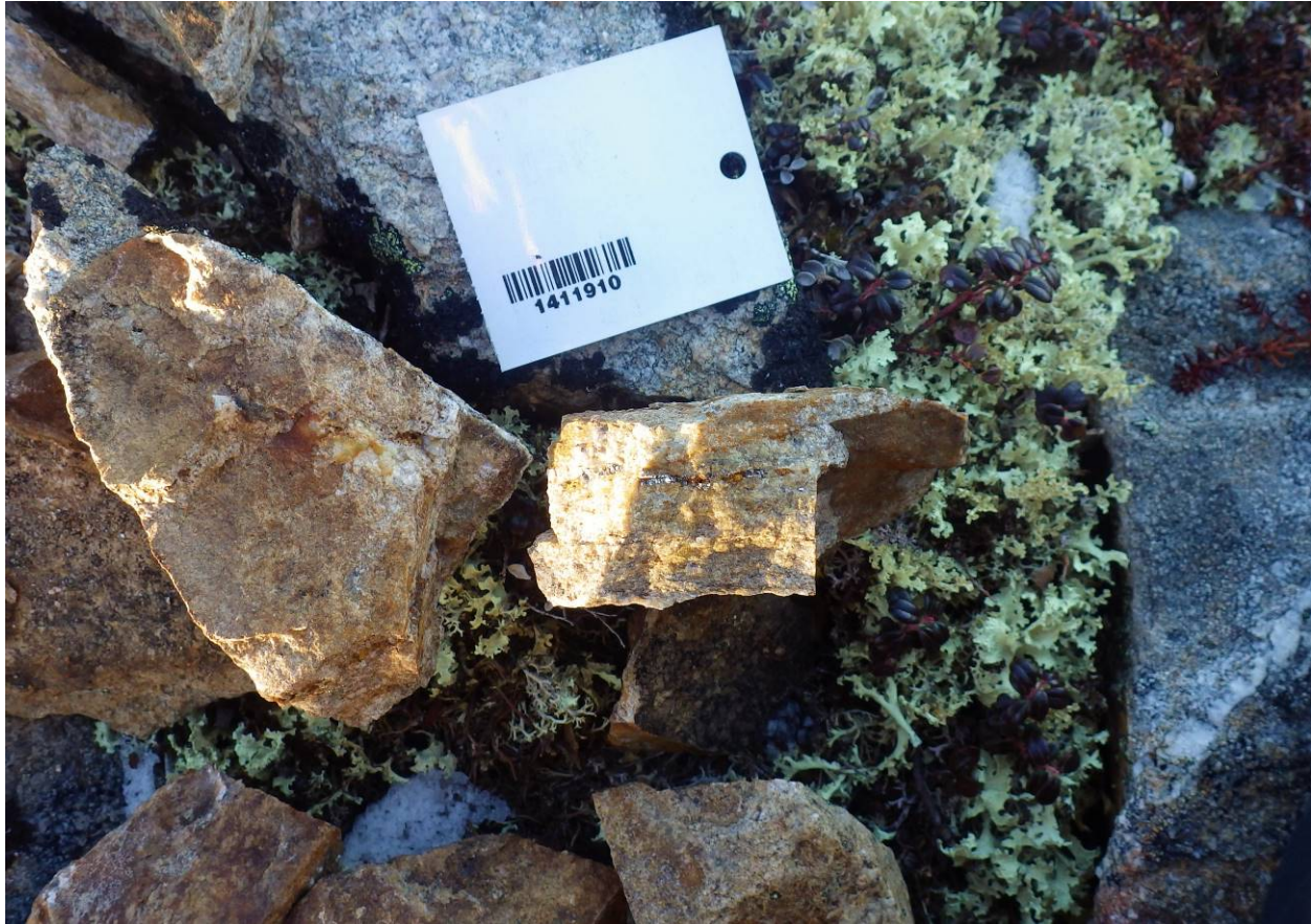
Figure 26: Quartz-sericite altered felsic gneiss from the Skye Zone with quartz veining and foliation parallel pyrite. Sample assayed 0.157 g/t Au.
