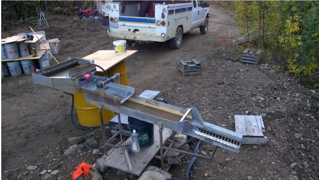
Photo 2: Gimlex drill sample Long tom with finger grizzly expanded metal and angle iron riffles used for processing samples.
