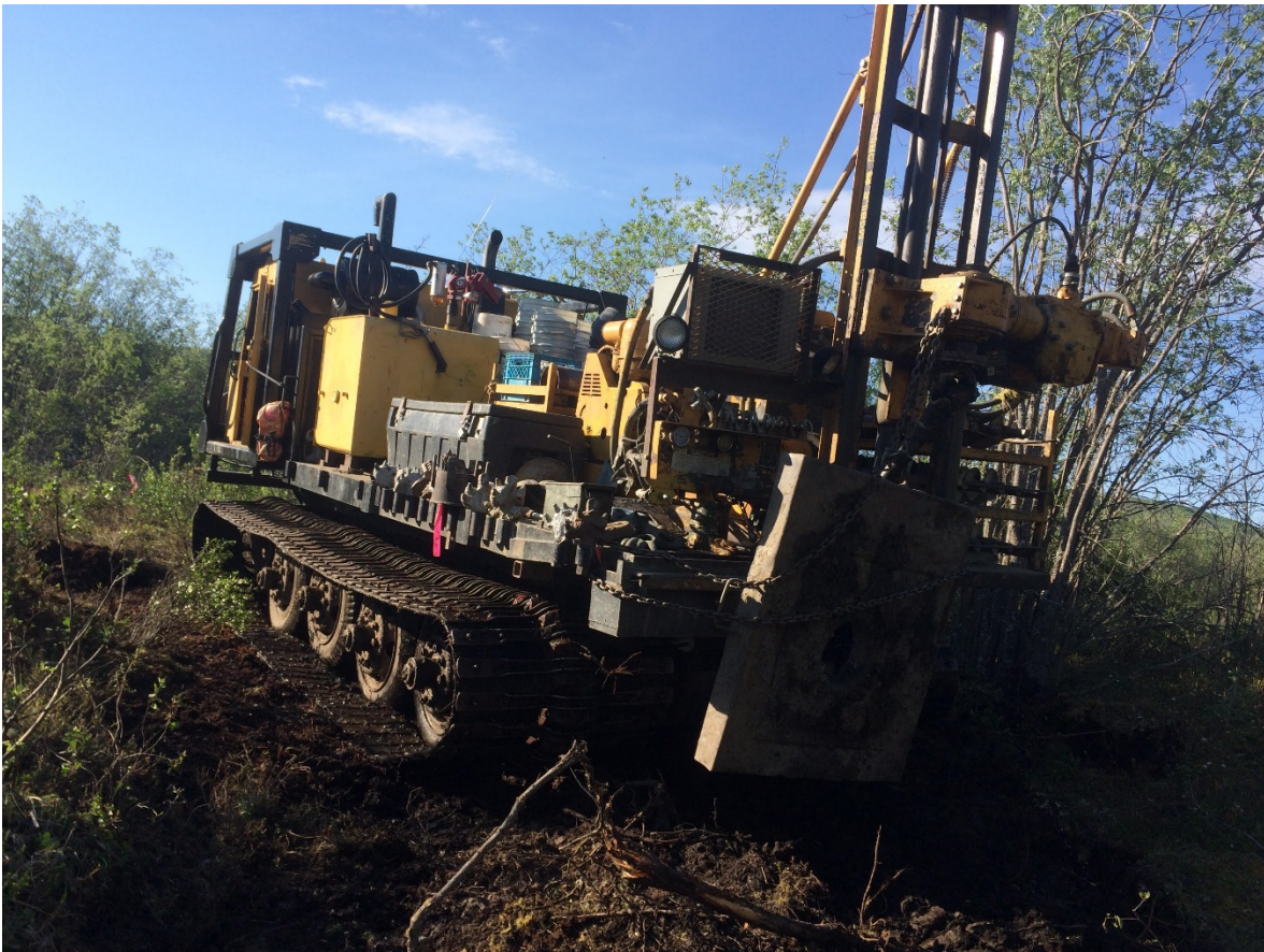
Photo 1: Gimlex's B31 Drill mounted on FN110 Nodwell carrier.
