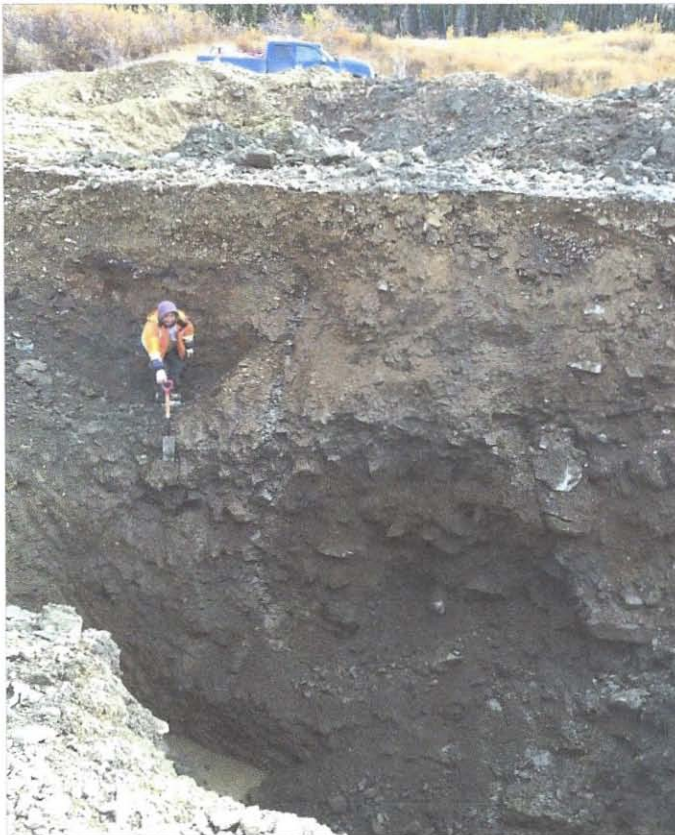
Figure 4 The Test Pit, Showing the Auriferous Glacial Till Sediments (After Dr. Y.T. Guo, P.Geo., 2016)
