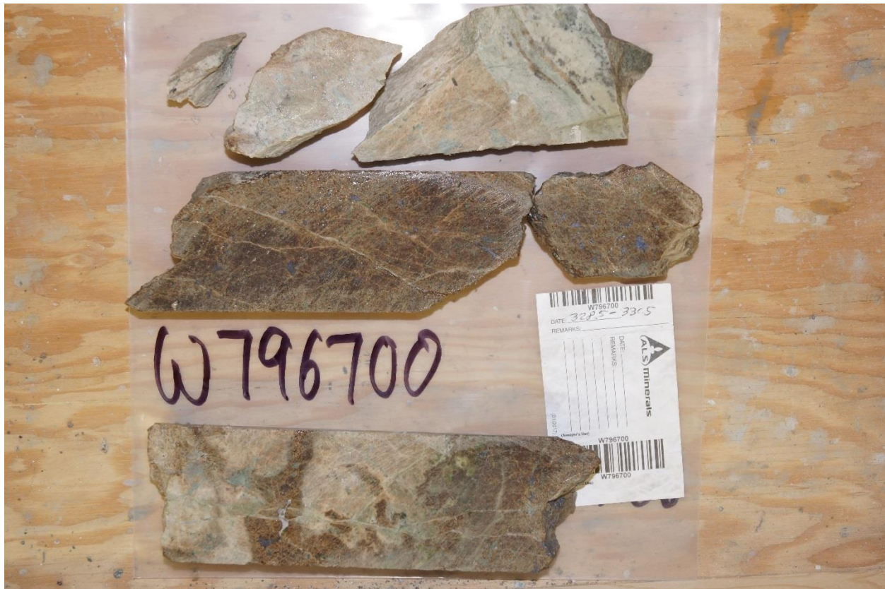
Photo 1. Sample W796700, coarse disseminated interstitial molybdenum, 0.8% Mo over 2 feet.
