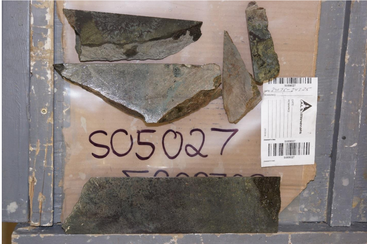
Photo 5. S057237 strongly mineralized skarn with semi-massive chalcopyrite-bornite assaying 8.34 % Cu, 0.92 g/t Au and 55.3 g/t Ag over 1.5 feet.
