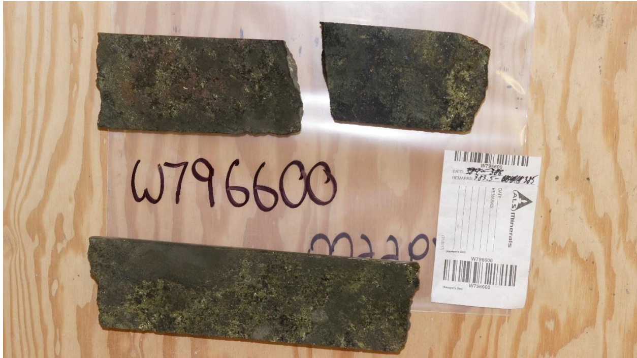
Photo 3. W796600 strongly mineralized skarn with semi-massive chalcopyrite-pyrite assaying 12.35% Cu over 1.5 feet.
