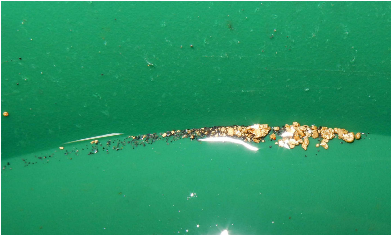
Figure 9 - Gold from sample S-3 (Test Pit 2016-11) on the Stuart claims tributary was a mixture of coarse to medium colours, and weighed approximately 100 mg. The sample volume was 7.64 cubic metres.
