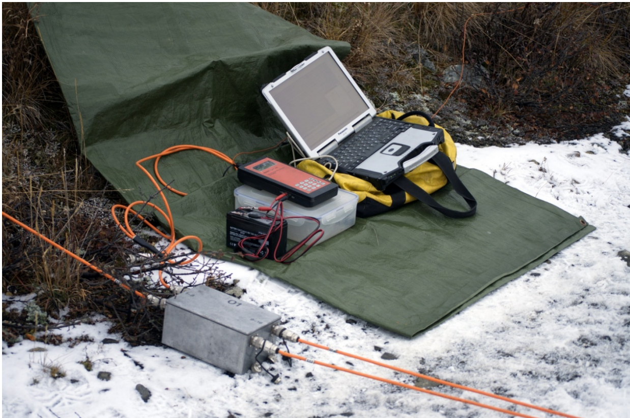
Resistivity/IP measurement, Stefan Ostermaier, Arctic Geophysics Inc., Atlin, BC 2013
