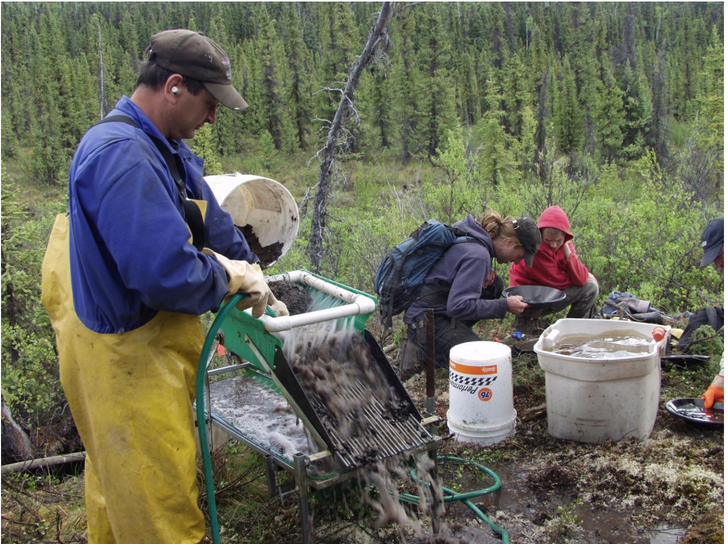
Photo 1 - During the 2003 auger drilling program, drill samples were processed in the field using a Le Trap long tom. Concentrates were then panned and the gold dried and weighed. The highest grade samples contained 181 mg Au (drill hole 2003DH07) and 117 mg Au (drill hole 2003DH04) respectively.
