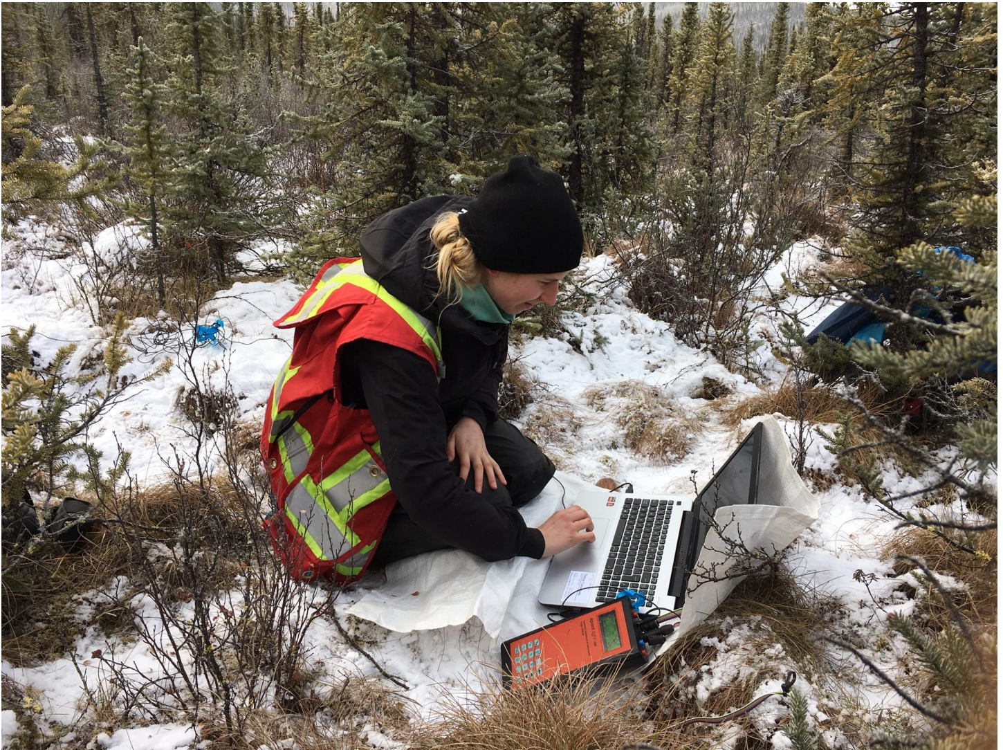
Photo 2 - Data was captured in the field using a laptop running the Geotest and RES2DINV programs, and the Lippmann 4 point light resistivity meter. Moderate snow conditions and below freezing temperatures required some additional time and care in deploying the geophysical equipment.
