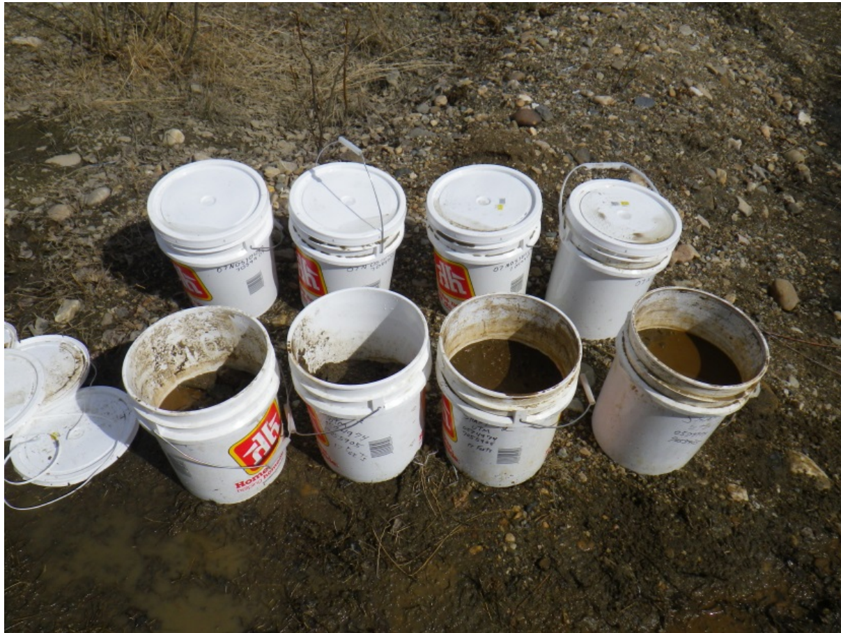
Figure 9: Reindeer shaft samples in new pails, each labelled and sealed for security.
