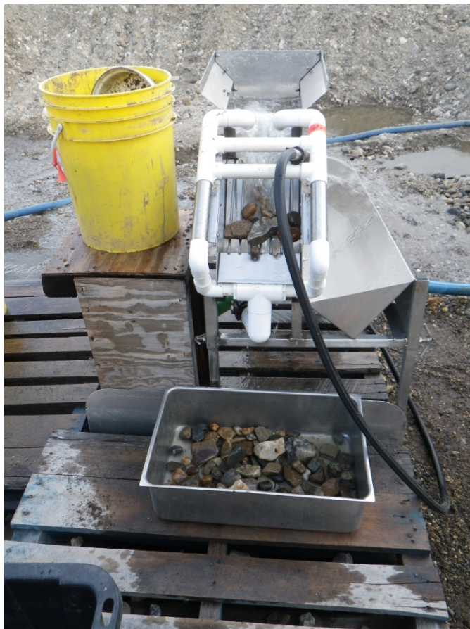
Figure 11: Oversize material is collected in a pan below the grizzly.
