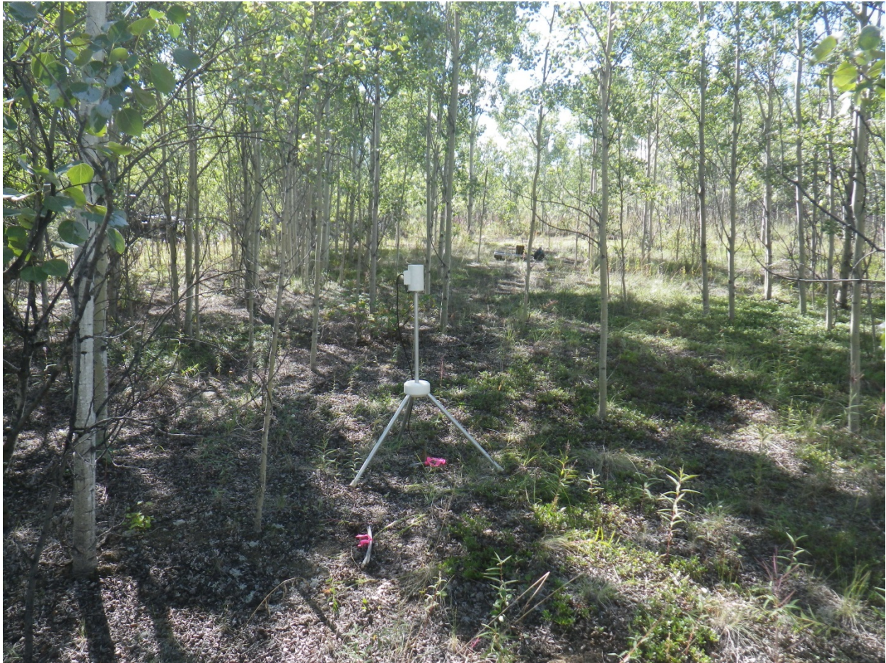
Figure 19: Base Station sensor on tripod and magnetometer set 20m away on Haystack Bench.
