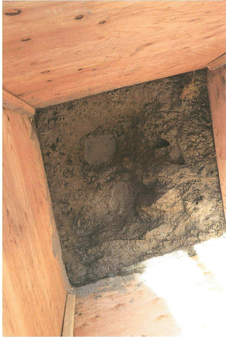
6 FOOT LEVEL NOTE: HARD BLOCKY BEDROCK ON RIGHT
