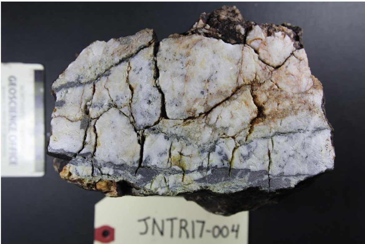
Figure 2: Hand sample cut surface showing quartz clasts (white) with arsenopyrite-scorodite veining (black)
