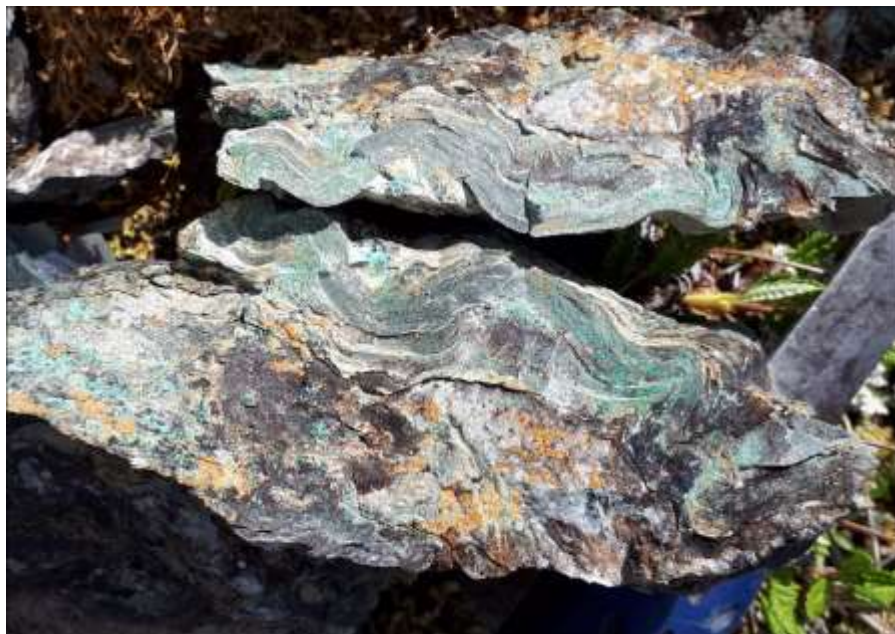
Photo 2 Rock sample I065266, folded silty phyllite with quartz, carbonate sericite alteration, blabs and spotted chalcopyrite and pyrite 1-2%. Assay return Cu, 4690 ppm, Au, 0.09 g/t, Ag 1.02 g/t.
