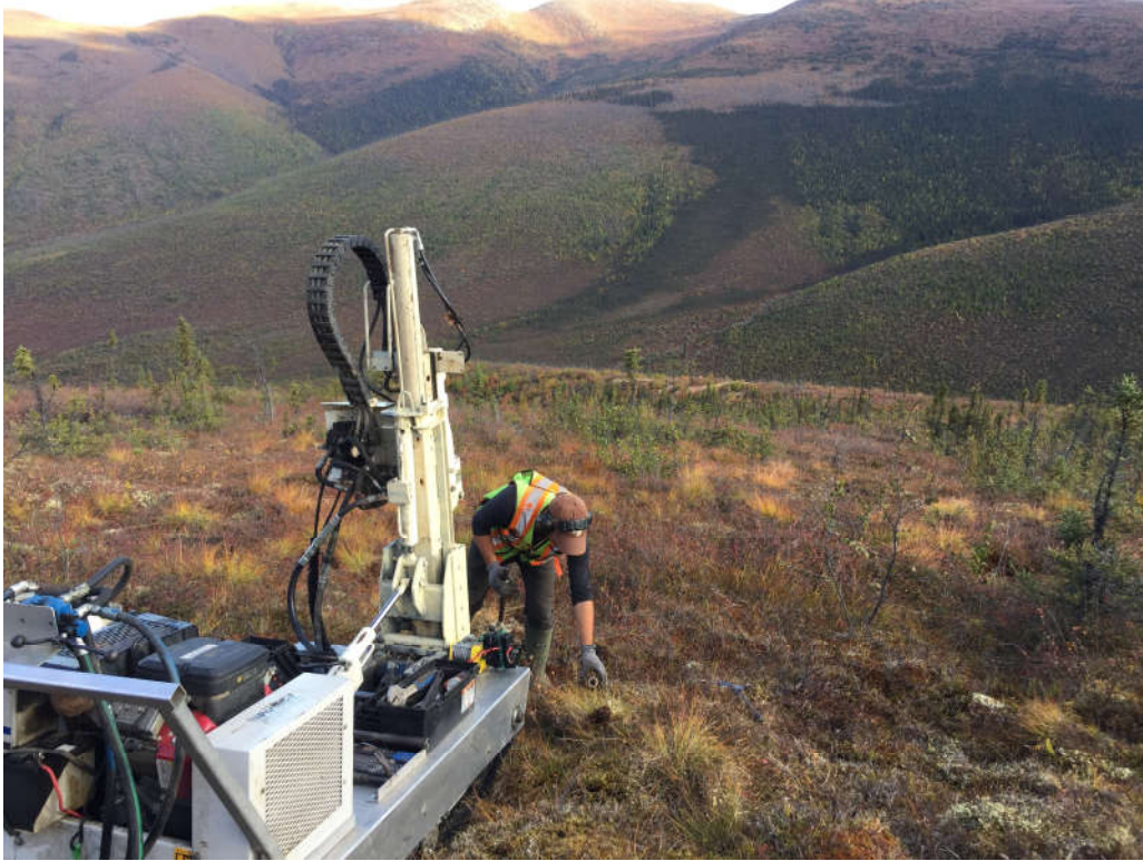
Photo 4: Geoprobe sampling on Big Creek target.
