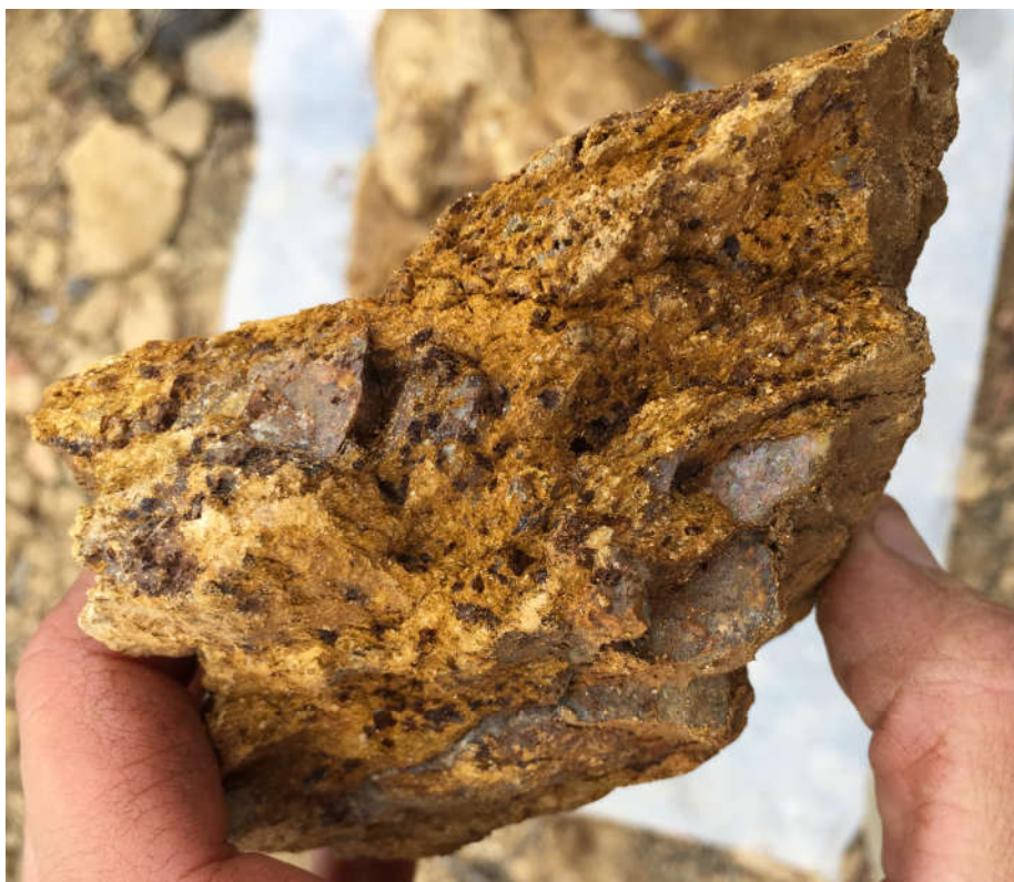
Photo 1: Pyritiferous and oxidized rock sample W641310 assayed 43 ppb Au and was anomalous in pathfinder elements.
