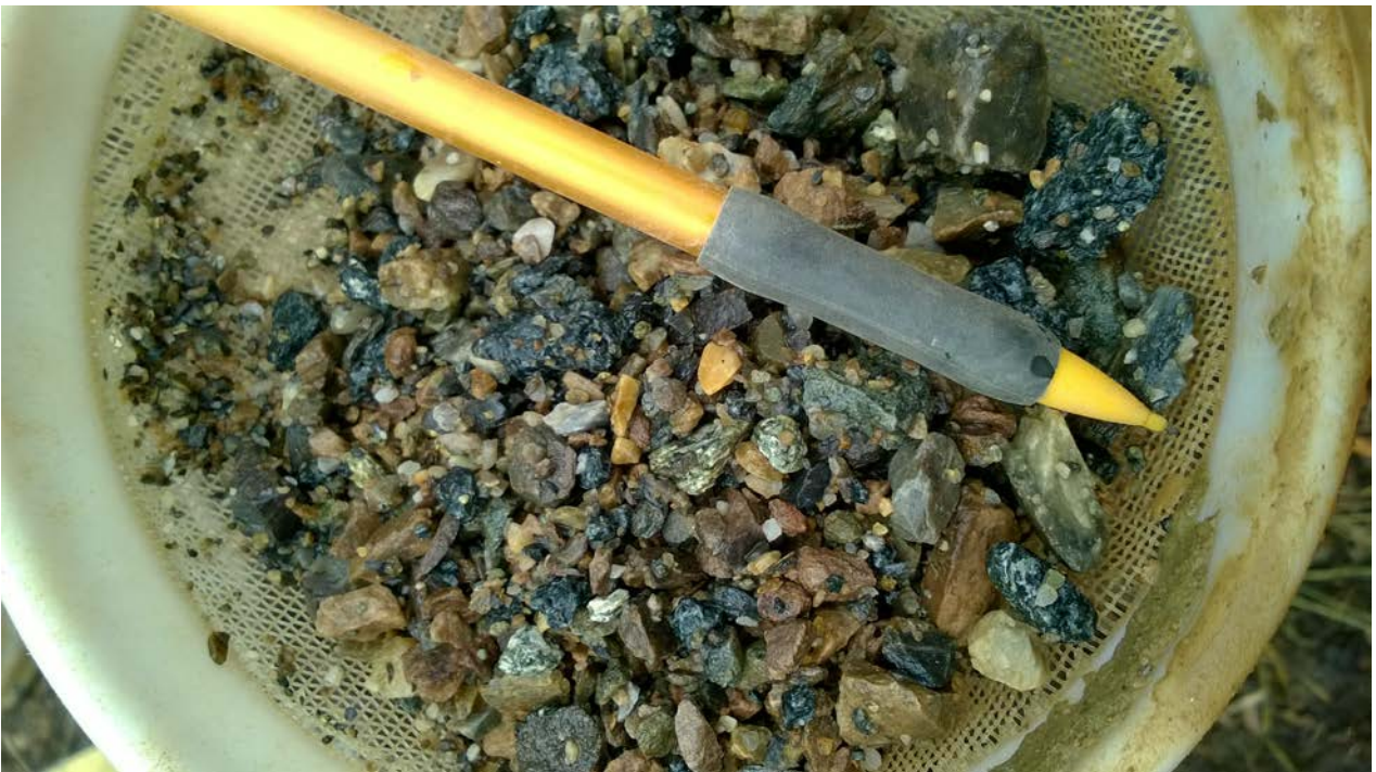
Figure 17: Geologists sieve sample RC rock chips at bedrock contact. Dark greenish grey chips are phyllite.
