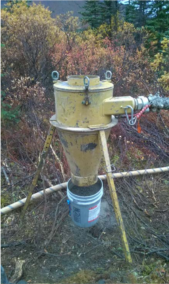
Figure 14: Dry sample collected under cyclone on Hole #6. (left)
