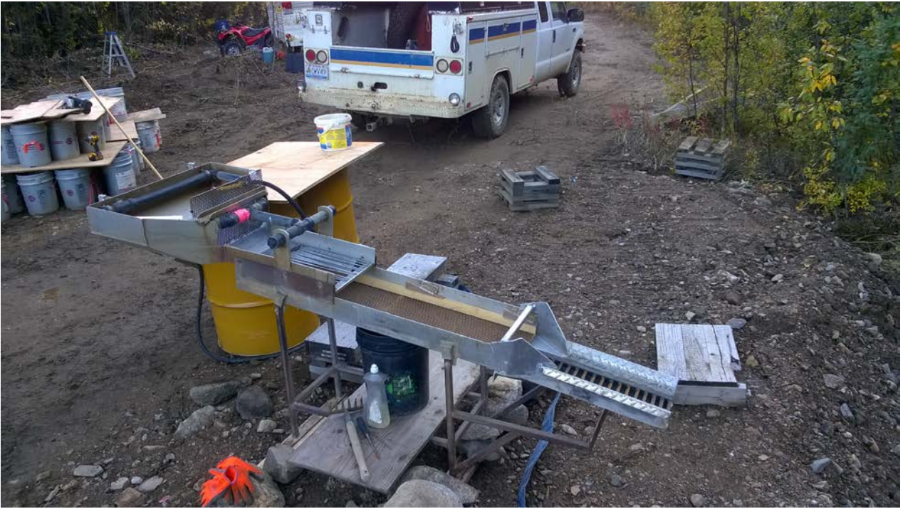
Figure 18: Longtom used to concentrate drill samples.
