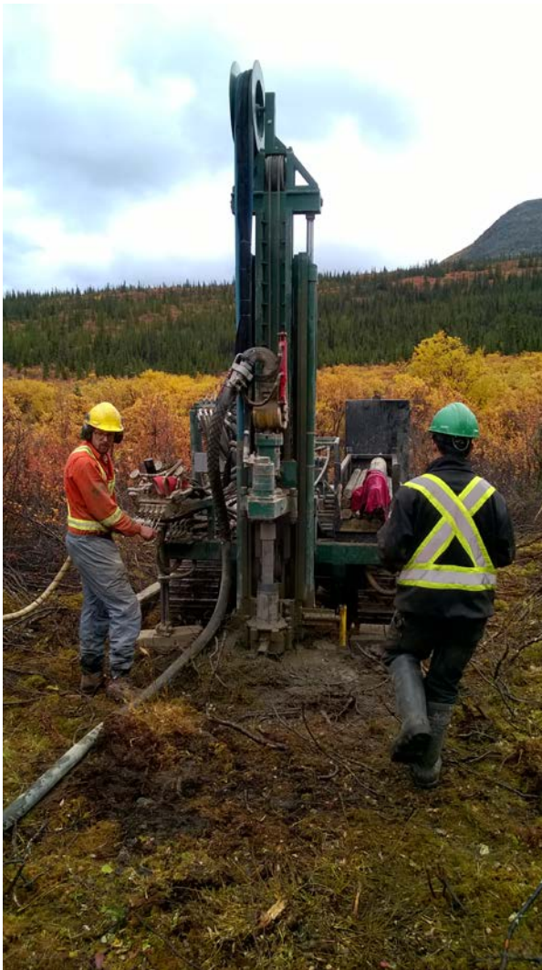
Figure 12: RC Drill, compressor and cyclone on Hole #6. (above)
