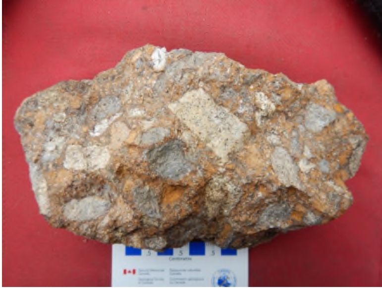
Figure 43. Fragmental volcanic rock (lapilli tuff or volcaniclastic pebble conglomerate) from Wind Zone trench (396447E, 6886497N, UTM Zone 08V, NAD83). Blue bars of scale card are 1cm wide.
