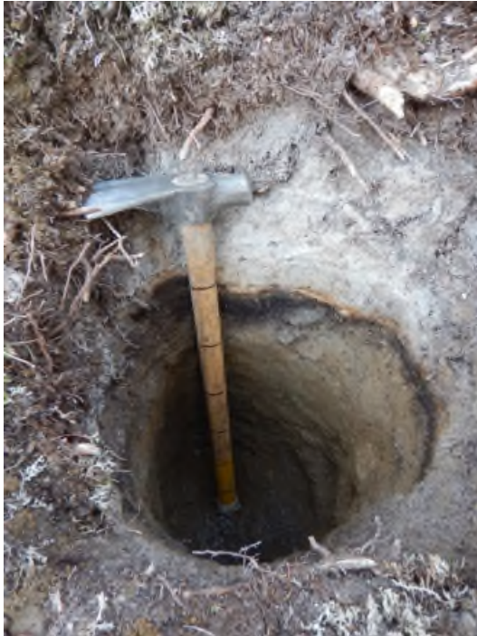
Figure 17. Soil pit DA2032 (393346E, 6884410N, UTM Zone 08V, NAD83). White, 22 cm thick layer of ash (near Geotul head) underlain by 5 cm black, organic-rich layer. Pit is 85 cm deep. Geotul handle is marked in 10 cm increments.
