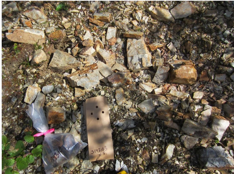
Plate 9: Sample S193103, from altered phyllitic quartzite with abundant iron and manganese oxides in fractures. Sample taken from roadcut near the western margin of the Bighorn Soil Anomaly (454065E/7084252N). No historical work has been recorded in this area.
