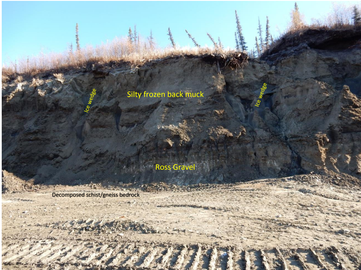
Figure 20 – View of the pit wall looking east towards the left limit, Sept 28, 2018. The 5 ft. thick white-grey gravel at the base of the section is likely the "Ross Gravel", which at 780,000 years B.P. is older than the overlying Sulphur Creek gravel.
