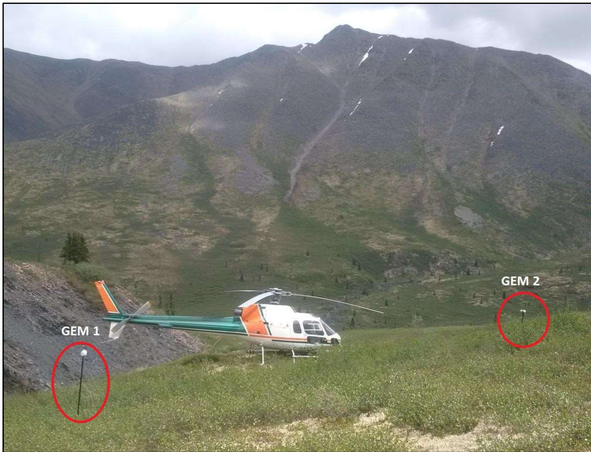
Figure 8: GEM 1 (left) and GEM 2 (right) magnetic base stations at the Monster survey block.
