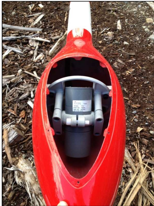
Figure 15: View of cesium vapor magnetometer. Sensor oriented 45° from vertical to couple with local magnetic field at the Monster survey block.
