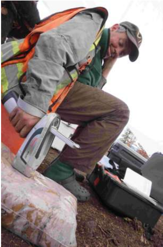
Testing soils by XRF each evening
