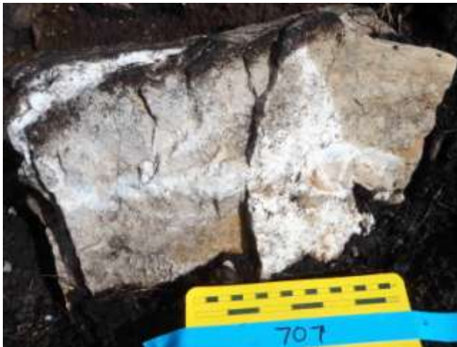
Typical quartz veins tested by XRF at the STEW project.
