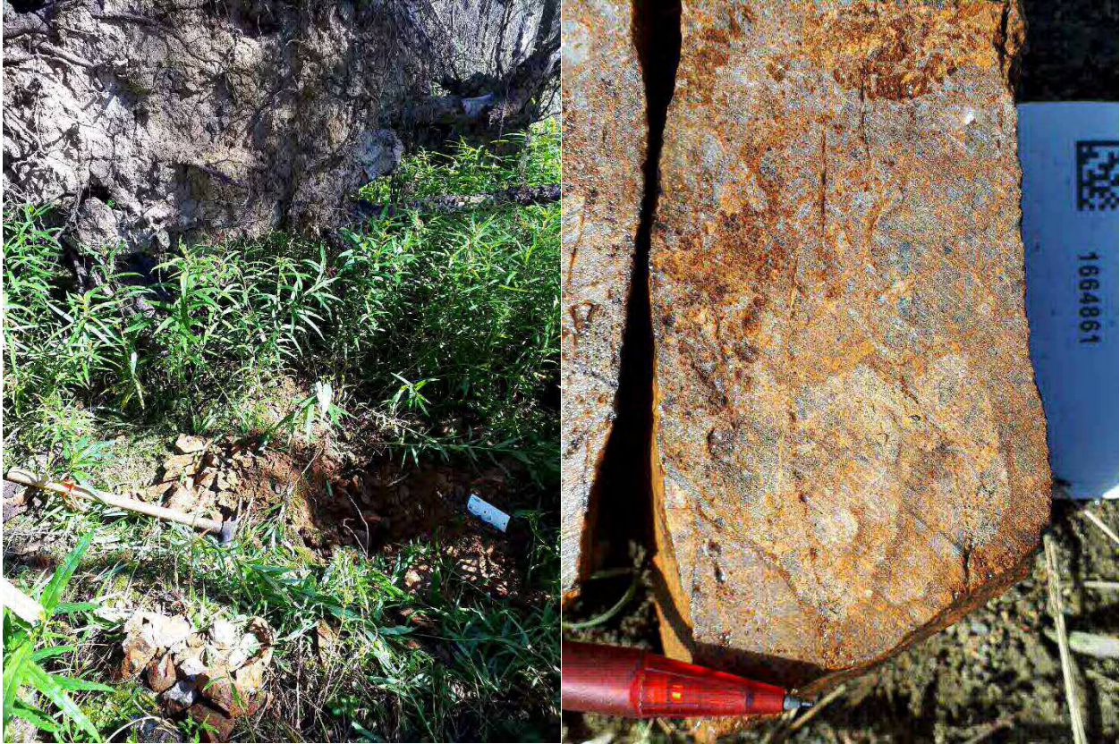
Figure 14. Abundant sericite and silica altered felsic gneiss found beneath a fallen tree roots. Pervasive limonite stain and traces of finely disseminated Fe-oxide specs likely after relict pyrite. Sample 1664861.
