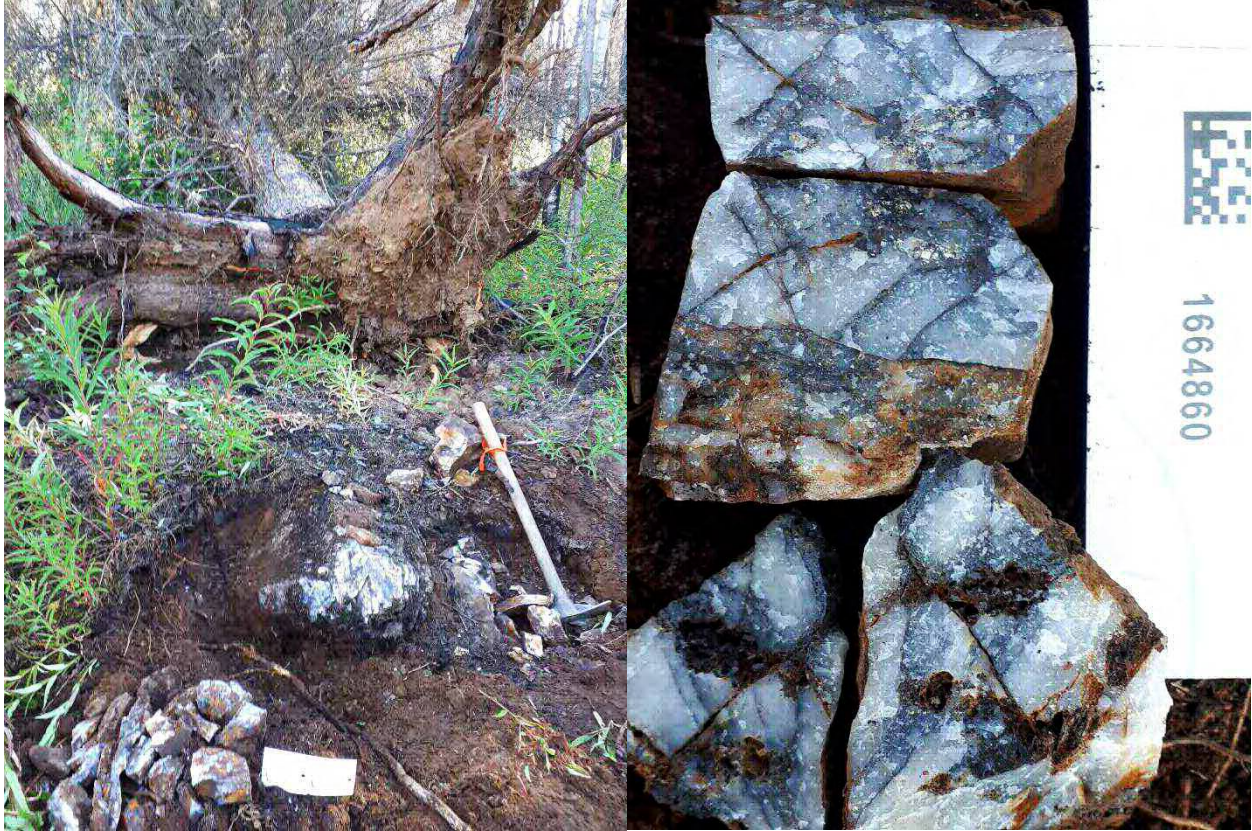
Figure 13. Quartz vein boulders exposed under a windfall tree. Intensely fractured vein quartz with specular hematite veinlets and coarse pyrite.
