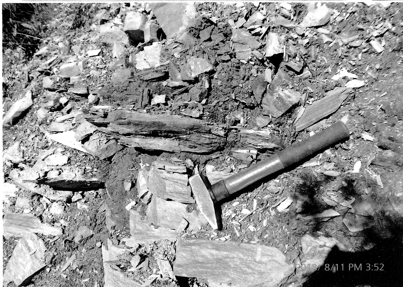
WP403 PUP 2 oxidized chlorite schist at base of talus slope – 107ppb gold
