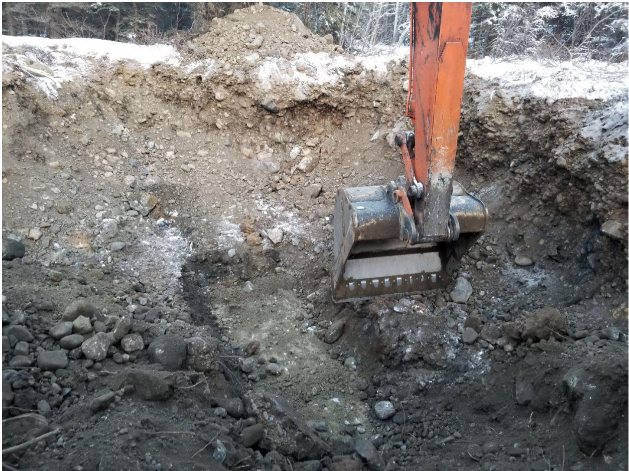
Plate 2 – Test Pit 18-01 was excavated along Resistivity Line RES18-AIE-04. The stratigraphy consisted of 3 metres of gravel overlying a fine silt. Bedrock was not reached.
