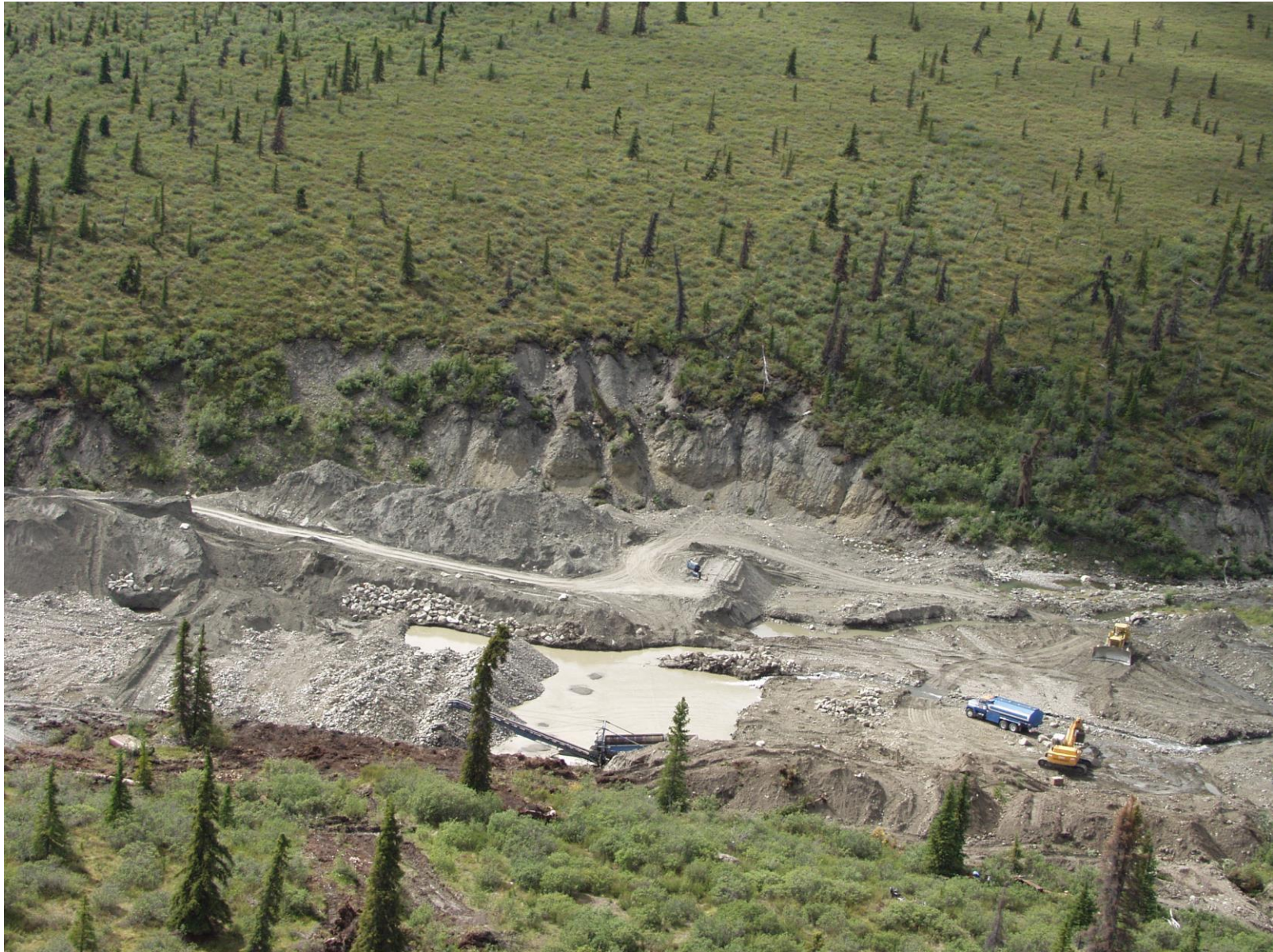
Plate 3 – Aerial view of the Sota Computing Ltd. operation on the left limit of Fourth of July Creek, 2002. The stratigraphic section was described (LeBarge, 2007) as mixed sand and gravel over a layer of glaciolacustrine silt and clay, which was overlying the pay gravel. Underlying the pay gravel was a unit characterized as a “false bedrock” of glacial till.
